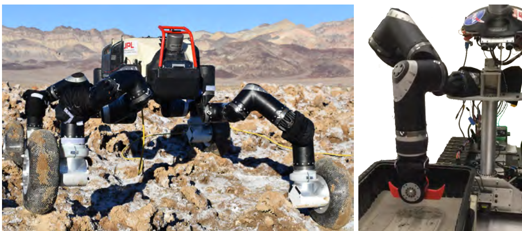
Figure 3.1: Left: JPL’s RoboSimian platform traversing rough Europa analog terrain in Death Valley, CA [111]. The platform possesses a total of 32 Degrees of Freedom (DoFs), spread across four articulated limbs with wheels at the distal joint. Right: JPL’s SURROGATE platform executing a “sweeping” excavation mode on regolith simulatant with a multi-tool mounted on 7 DoF limb.
