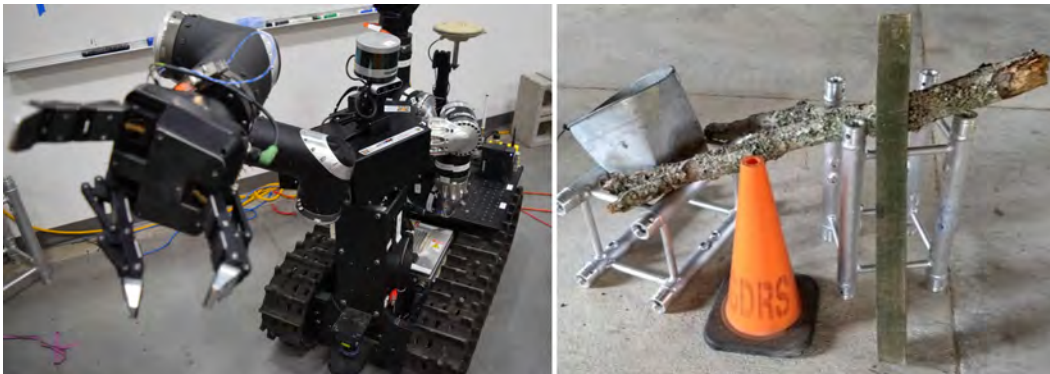
Figure 5.1: Left: Army Research Lab's 'RoMan' mobile manipulation platform with broken proximal joint on Robotiq 3-finger gripper. Right: Example debris pile of massive objects, where lifting two or more items simultaneously may exceed manipulator payload limits.
