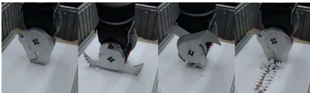
Figure 3.13: Action sequence of PIU-ED policy (left to right) for substrate step change in presence of operator preference for raking. [raking, sweeping, chomping, raking]
