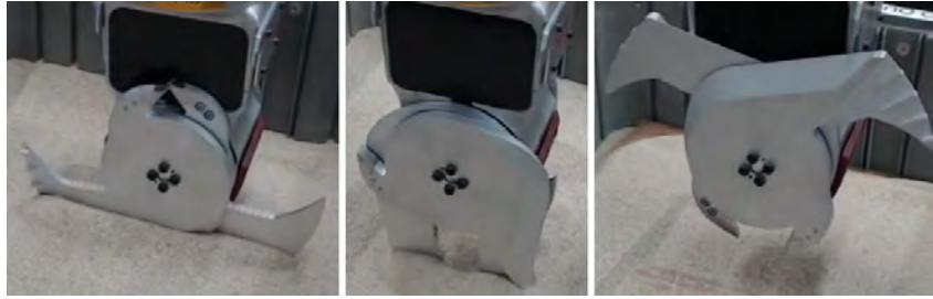
Figure 3.7: Three substrate excavation modes available on the SURROGATE multi-tool platform. Left: Sweeping mode with 20cm wide tool. Center: Raking mode with 8cm wide oscillating tool. Right: “Chomping” mode with two steel teeth engaging surface 8cm apart.
