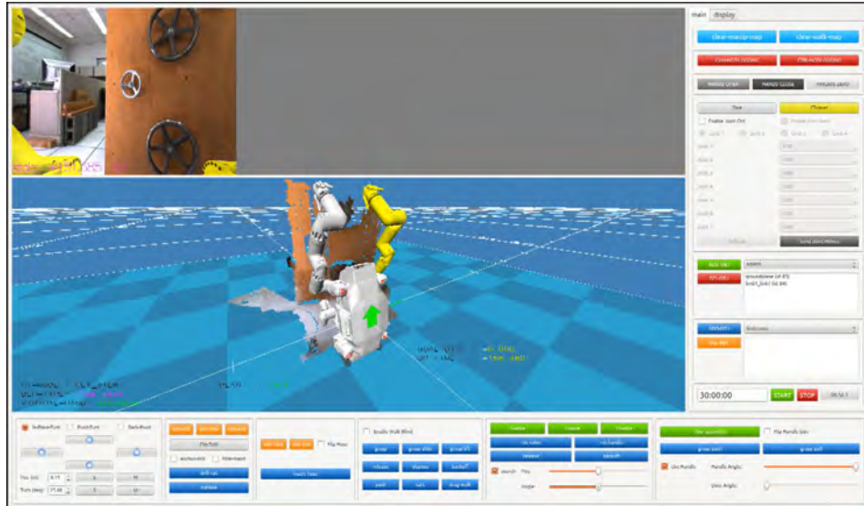
Figure 1.4: Operator panel used during DRC trials for valve turning task
