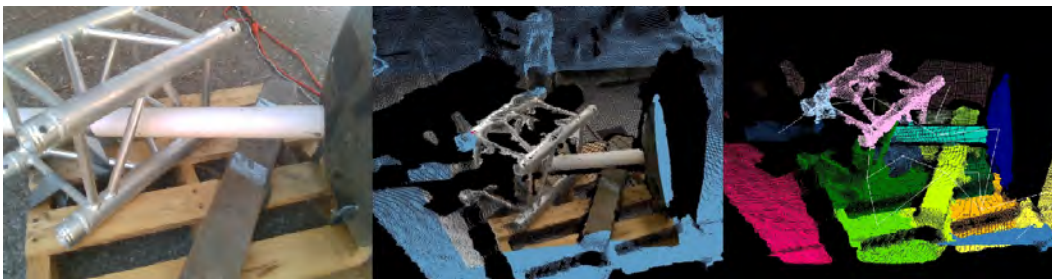
Figure 5.2: Left: RGB image of example debris pile containing aluminum truss segment, safety barrier, 4x4 wood section, and pallet. Center: Point cloud of workspace captured with RealSense D435. Right: Singulated object candidates with geometric adjacency from Locally Convex Connected Patches algorithm. [127]
