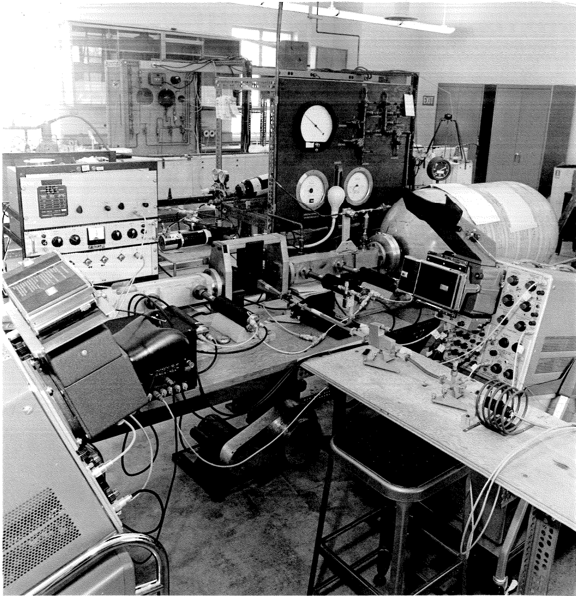
Fig. 3. A View of the Diagnostics Section of the Shock Tube
