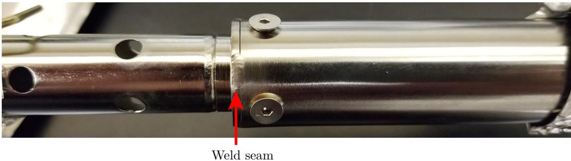
Figure 7.8.2: Photograph of the bolted sample probe interface after welding.
