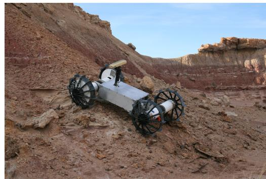
Figure 1.9: The DuAxel rover on rough terrain. DuAxel consists of two Axel-class rovers docked with a central module.
