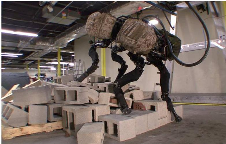
Figure 1.6: Even free-standing robots often use a tether during testing, for power or safety. Big Dog, a quadruped robot by Boston Dynamics, is shown here with a cable [46].
