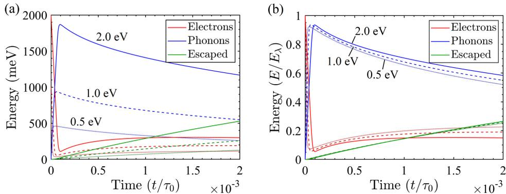
Figure 2.3: Simulated downconversion with NbN material parameters for (a) various photon energies. The energy was distributed as a single electron-hole pair for 0.5 eV (dotted), 1 eV (dashed), and 2 eV (solid) photon energies. The initial downconversion timescale is slower for higher energy photons. (b) When normalized by the photon energy, it is clear that more energy remains in the phonon system as the system thermalizes for higher energy photons.
