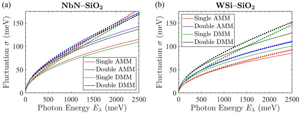
Figure 2.20: Fluctuations during downconversion for (a) NbN and (b) WSi on SiO<sub>2</sub>. Circles indicate the calculation including the  $z$  contribution according to (2.52) while the lines show the  $\sim \sqrt{E_\lambda}$  dependence according to (2.51).
