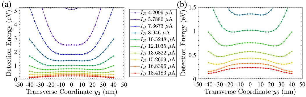
Figure 3.15: Detection energy as a function of transverse coordinate for a 100 nm wide wire at various bias currents. As the bias current increases, the detection energy decreases. A closer view (b) of the high bias current region shows the transition from a ‘W’ shape to a ‘Bell’ shape.
