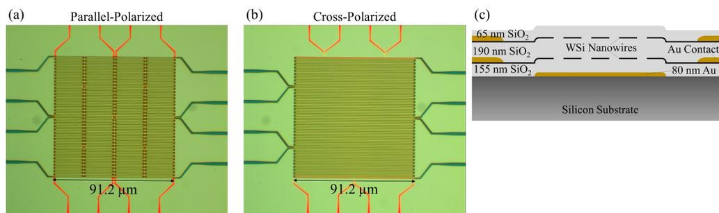
Figure 5.2: Optical microscope images of (a) parallel-polarized and (b) cross-polarized devices. Blue channels are the top layer while red channels are the bottom layer. (c) Schematic cross-section of the TRC devices showing layer thicknesses.
