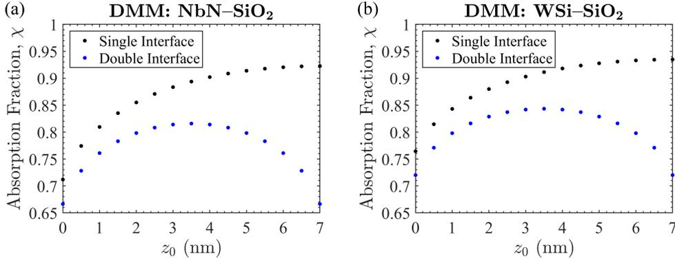
Figure 2.19: Average absorbed energy for (a) NbN and (b) WSi on  $\text{SiO}_2$  within the framework of the DMM. Black indicates the case of a single interface with the substrate material while blue indicates a double interface.
