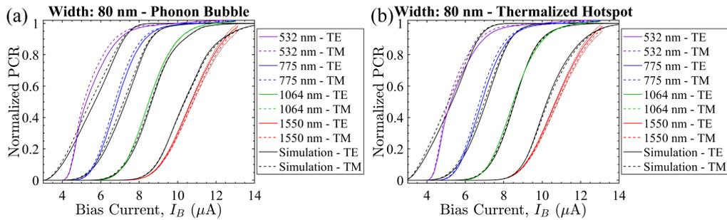
Figure 3.24: Comparison of model fitting for (a) phonon bubble initial conditions and (b) thermalized hotspot initial conditions.
