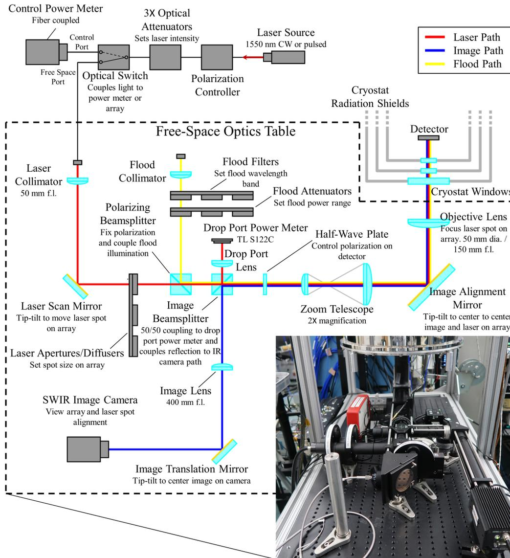
Figure 6.3: Optics system diagram. Black lines indicate optical fiber connections while the colored lines indicate the free-space beampath. When the breadboard is moved from underneath the cryostat, a power meter is mounted at the focal point of the objective lens to calibrate the transmission of the free space optics system (not shown). A picture of the free-space optics is shown for reference.
