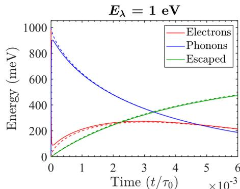
Figure 2.13: Comparison of downconversion calculations using the electron bubble (solid lines) and phonon plateau (dashed lines) initial conditions with diffusion included while using the cylindrical coordinate system. There is a larger difference between the two initial conditions when diffusion is included compared to the fixed hotspot results, but the agreement is still good.
