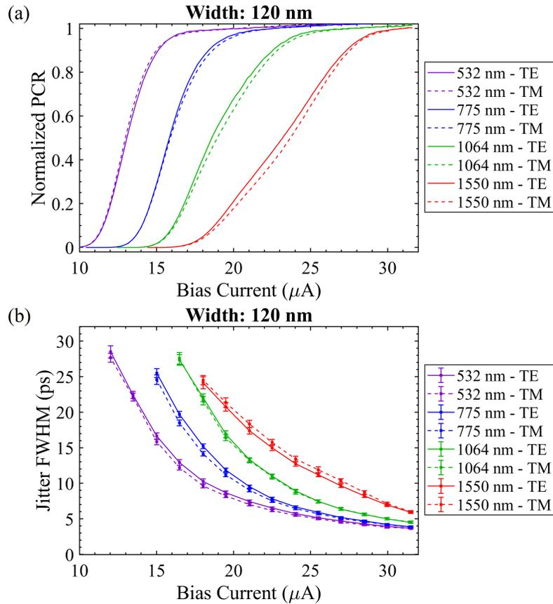
Figure 3.5: Polarization-dependent (a) PCR and (b) timing jitter for a 120 nm NbN device measured at a bath temperature of 1 K. Solid lines indicate the TE polarization and dashed lines show the TM polarization.
