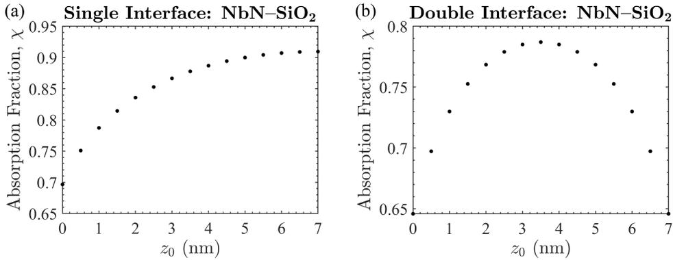
Figure 2.17: Average absorbed energy fraction in a NbN nanowire on SiO<sub>2</sub> for a (a) single interface and (b) double interface using the AMM.
