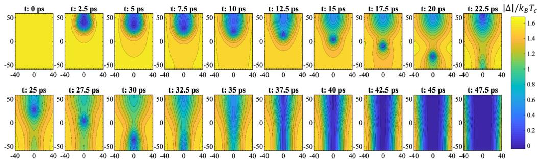
Figure 3.11: Evolution of the magnitude of the order parameter for a detection near the edge of a 120 nm wire. The vertical scale is the transverse coordinate  $y$  while the horizontal scale is the longitudinal coordinate  $x$  with the bias current flowing from left to right. The formation and subsequent motion of single vortices from one edge to another facilitates the suppression of superconductivity.
