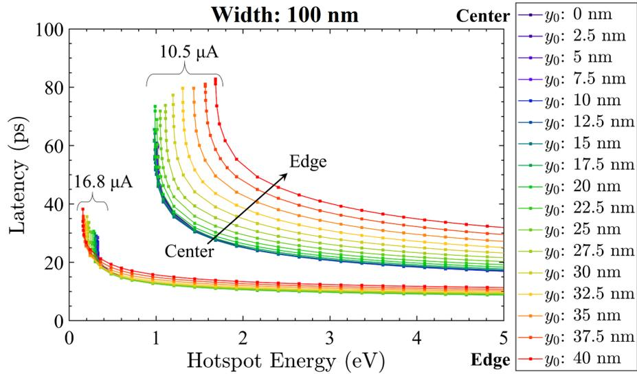
Figure 3.14: Simulated latency for bias currents of 10.5  $\mu\text{A}$  (upper family of curves) and 16.8  $\mu\text{A}$  (lower family of curves) for a 100 nm wide NbN nanowire.
