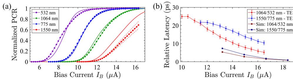
Figure 3.17: Comparison of the (a) PCR and (b) relative latency results of the Vodolazov TDGL model with experiment for the case of a 100 nm wide NbN detector operating at 4 K using a modified  $\tau_{esc}$  of 94 ps. The fitting parameters are  $\bar{\chi} = 0.44$  and  $\sigma_F = 96$  meV.
