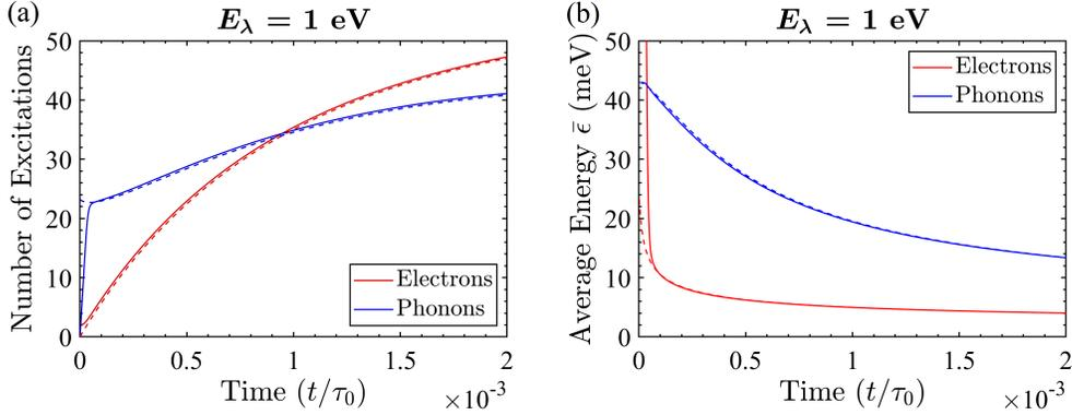
Figure 2.11: Comparison of downconversion calculations using the electron bubble (solid lines) and phonon plateau (dashed lines) initial conditions for a photon energy of 1 eV. The average number of excitations is shown in (a) while the average excitation energy is shown in (b).
