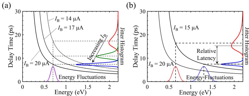
Figure 3.7: Connection between energy fluctuations and latency. For latency curves with different slopes (a), if the magnitude of the slope is larger, the magnitude of the jitter will also be larger for a given energy fluctuation distribution. For a given latency curve (b), increasing the photon energy leads to smaller jitter and a shorter delay time, resulting in a relative latency which can be measured experimentally.
