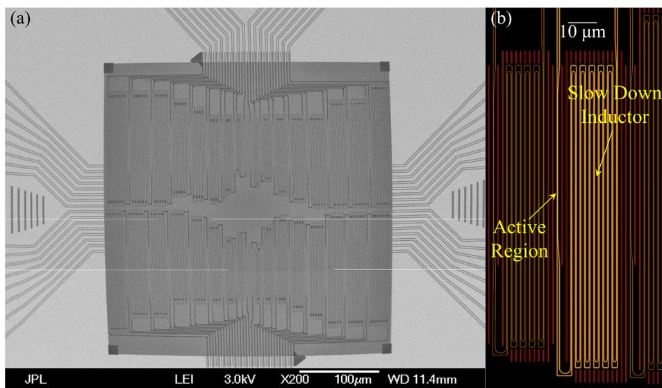
Figure 4.3: (a) SEM image of the latching devices fabricated to probe the reset characteristics of WSi nanowires. Each channel had a different length series inductor which controlled the reset time of the pixel. (b) CAD image highlighting a single pixel of the latching design. Each pixel consisted of a  $50\ \mu\text{m}$  long active segment with a wider series inductor.
