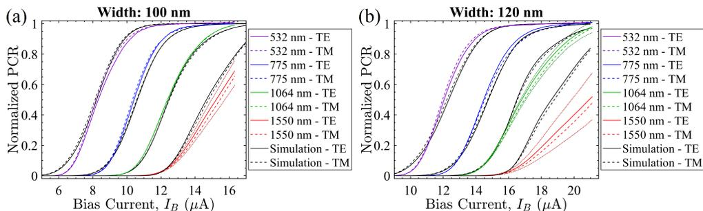
Figure 3.22: Comparison of simulated and experimental PCR curves for device widths of (a) 100 nm and (b) 120 nm. The colored curves are the experimental measurements while the black curves are the fit using the model. The dotted red and green curves show the approximate error bounds of the PCR curves for the 1550 nm and 1064 nm wavelengths, respectively. Solid lines indicate the TE polarization while dashed lines are the TM polarization.
