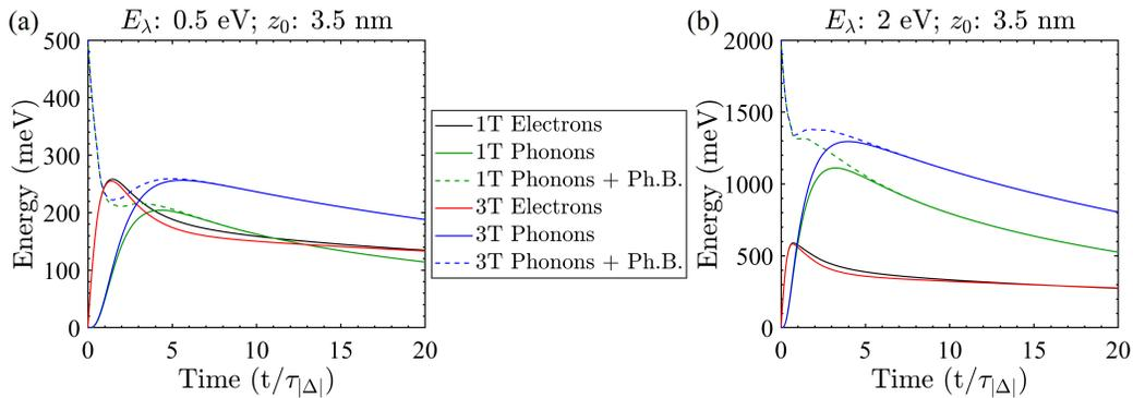
Figure 2.23: Comparison of the one-temperature and three-temperature models of WSi for a (a) 0.5 eV and (b) 2 eV photon energies. The separation of the phonon system into escaping and bottlenecked groups reduces the discrepancy between the two models at longer times, but there is still a deviation in the electron energy immediately after the electron system achieves its maximum energy.
