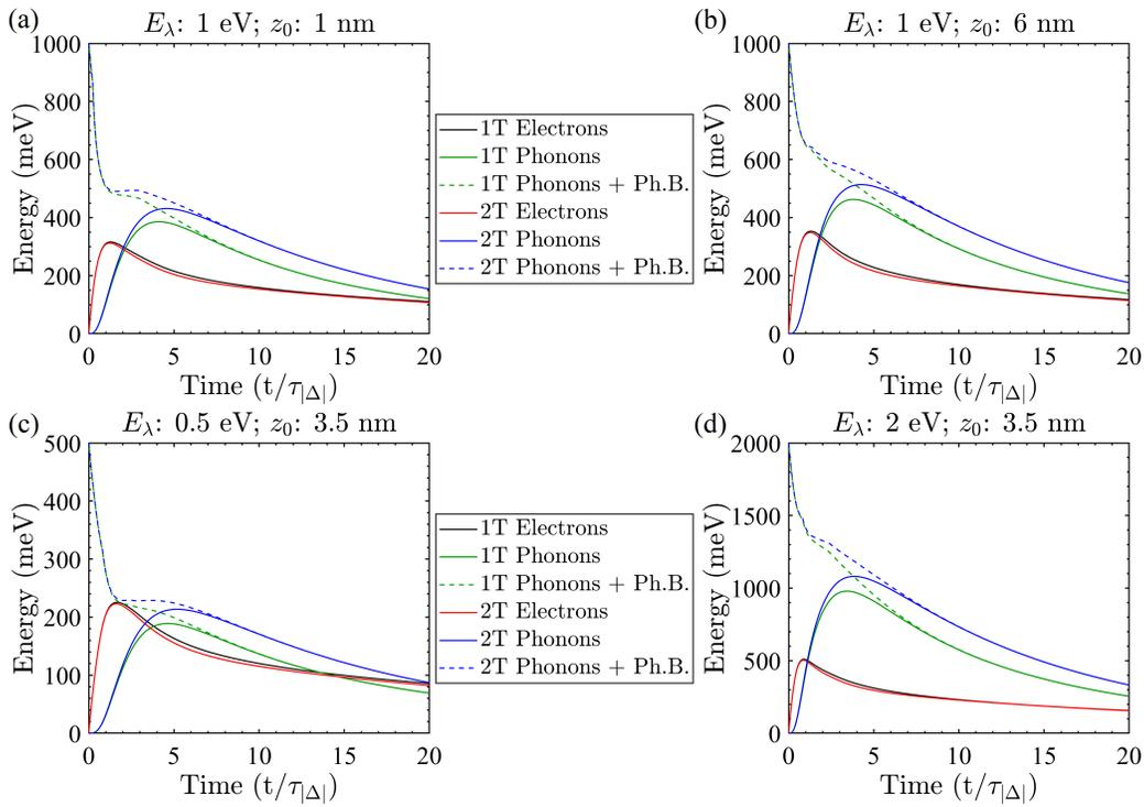
Figure 2.21: Comparison of the one-temperature and two-temperature models of NbN for a 1 eV photon energy at different absorption locations (a)  $z_0 = 1 \text{ nm}$  and (b)  $z_0 = 6 \text{ nm}$ , and different photon energies of (c) 0.5 eV and (d) 2 eV. The electron energies are comparable, but there are deviations in the phonon energies.
