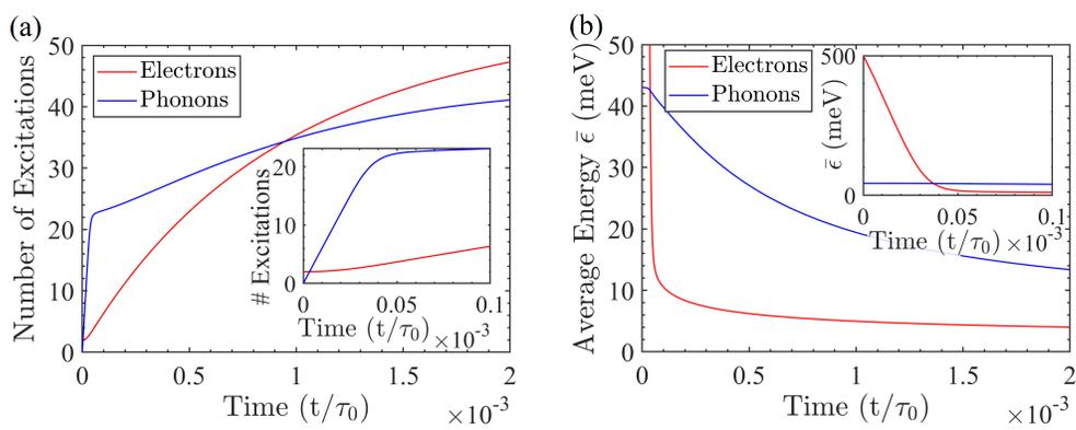
Figure 2.5: (a) Average number of excitations during downconversion using NbN material parameters. The inset shows the initial moments of downconversion and the linear rise in phonon number as the high-energy electrons couple to all phonon modes equally. (b) Average energy per excitation. The initial average phonon energy is 43 meV as predicted by (2.14). The inset shows the initial linear drop in electron energy on the same timescale as the number of phonon excitations increases.
