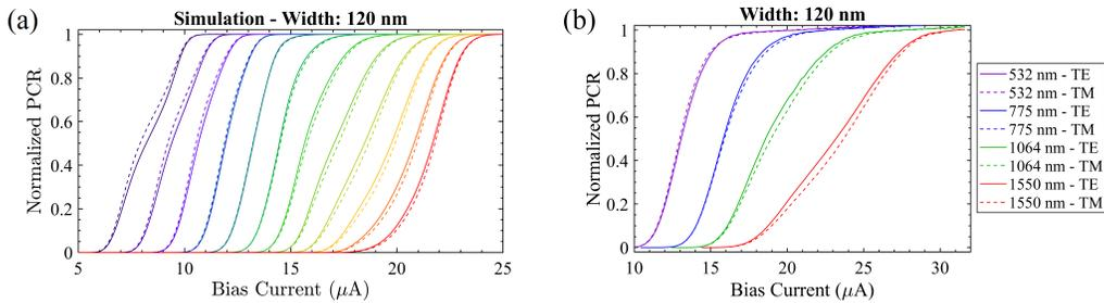
Figure 3.18: Comparison of polarization-dependent response of the Vodolazov TDGL model (a) with experiment (b) for the case of a 120 nm wide NbN detector operating at 4 K. Solid lines indicate the TE polarization while dashed lines are the TM polarization. The simulation parameters are  $\gamma = 40$  and  $\tau_{esc} = 30$  ps.
