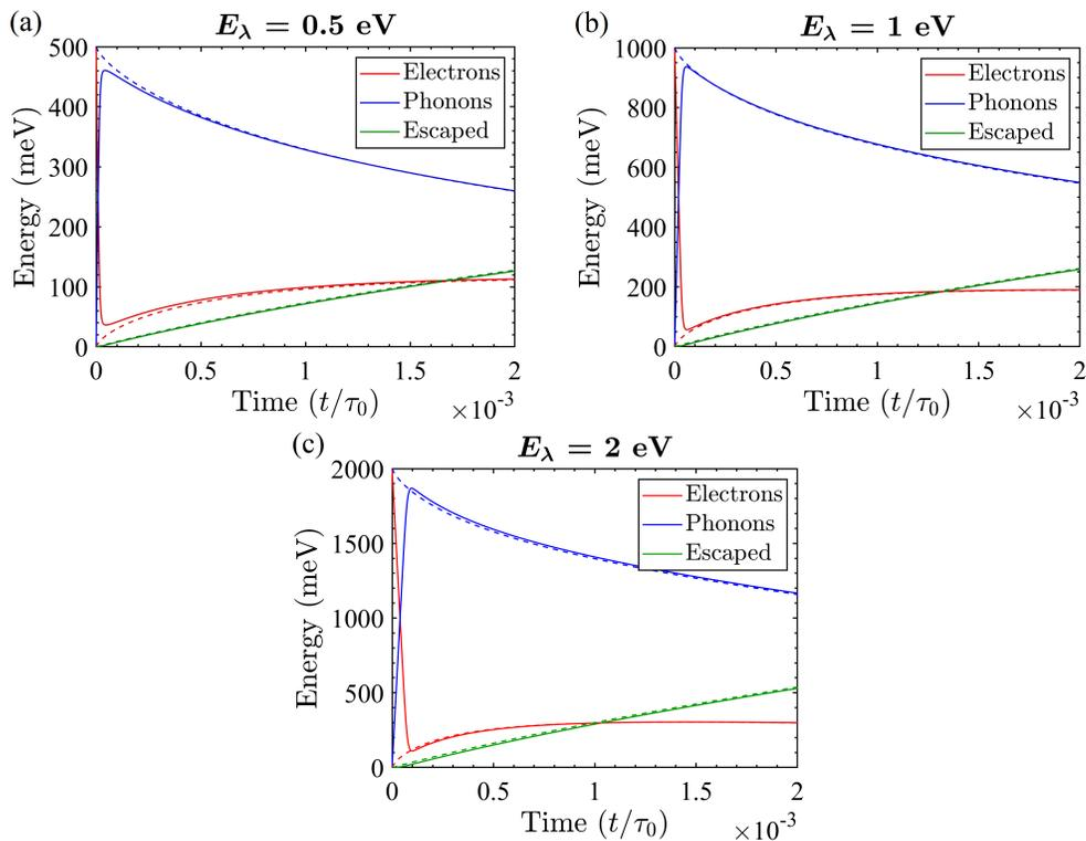
Figure 2.10: Comparison of downconversion calculations using the electron bubble (solid lines) and phonon plateau (dashed lines) initial conditions for photon energies of (a) 0.5 eV, (b) 1 eV, and (c) 2 eV.
