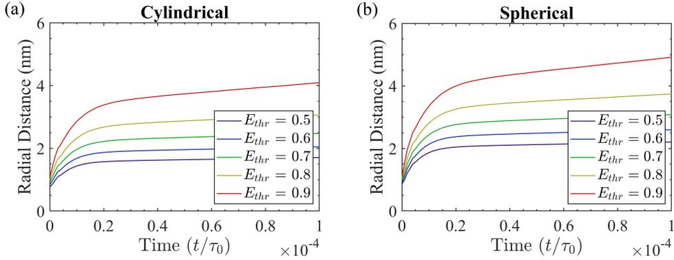
Figure 2.7: Radial distance containing certain fractions of the photon energy as a function of time for (a) cylindrical and (b) spherical coordinates.
