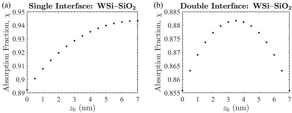
Figure 2.18: Average absorbed energy fraction in a WSi nanowire on  $\text{SiO}_2$  for a (a) single interface and (b) double interface using the AMM.
