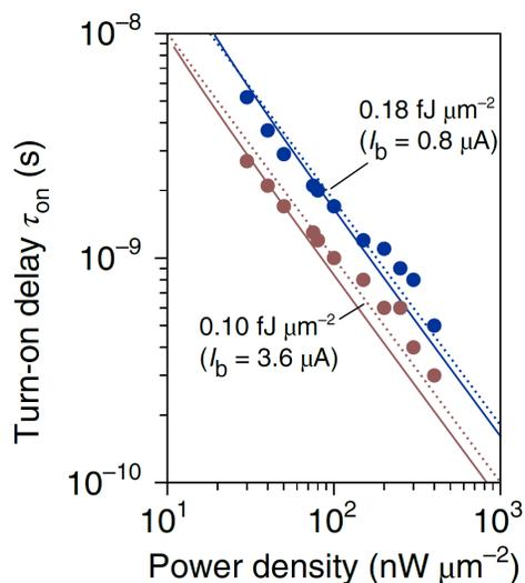
Figure 4.30: Turn-on delay for various applied power densities on the heater. The two colors represent different bias conditions on the superconductor. The solid lines are the fit using the ballistic transport model while the dashed lines correspond to curves of constant energy per unit area.
