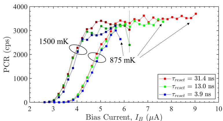
Figure 4.6: PCR measured at 1550 nm for three of the latching devices at 875 mK (light curves) and 1500 mK (dark curves). The emergence of saturated internal efficiency for the fastest device at higher bath temperature demonstrates a method of improving performance for devices which demonstrate latching. The dashed black line shows the switching current of the two slower devices at 1500 mK.
