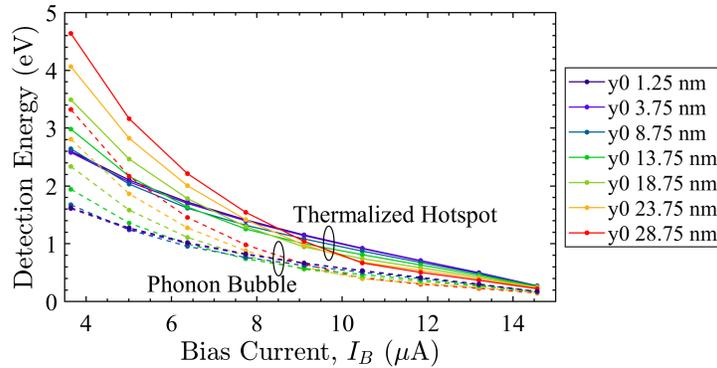
Figure 3.23: Comparison of the detection energy for the thermalized hotspot (solid lines) and modified phonon bubble (dashed lines) initial conditions for an 80 nm wide wire with the material parameters  $\tau_{esc} = 9.4$  ps,  $\gamma = 20$ , and  $\tau_{ee}(T_c) = 5$  ps.
