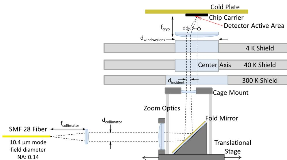
Figure 6.5: Schematic of the angled illumination experimental setup. Collimated light from a fiber was condensed to a small diameter collimated beam using a set of zoom optics mounted on x and y translation stages. This collimated beam entered the cryostat through the windows and was focused on the detector using a cryogenic lens. Translating the zoom optics changes the position where the collimated beam illuminates the cryogenic lens, which changes the angle of incidence at the detector.
