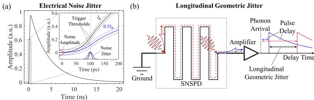
Figure 3.1: Jitter Overview. (a) Origin of the noise contribution to timing jitter. (b) Origin of the longitudinal geometric contribution to timing jitter. Differences in the distance microwave signals travel along the length of the SNSPD lead to different delay times in the onset of the detection pulse.
