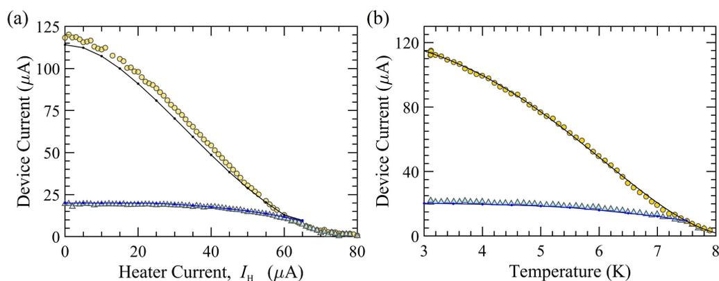
Figure 4.26: The switching current (yellow circles) and the hotspot current (blue triangles) of an M-hTron with a channel width of 600 nm and heater width of 500 nm as a function of (a) the heater current, and (b) temperature. The model predictions of the switching current (black line) and hotspot current (blue line) are shown for comparison. The model's temperature-dependent switching current is a fit to experiment.
