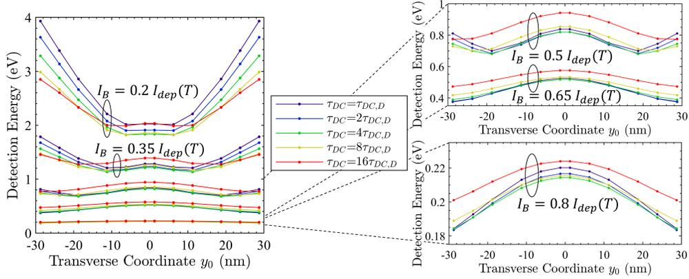
Figure 3.25: Simulated detection energy for various scaling factors to the value of  $\tau_{DC,D} = \frac{\tau_0}{\gamma\Omega_D}$ , which corresponds to the phonon-electron scattering time for Debye phonons. Colors indicate the correction factor, ranging from the nominal value (purple) to an increase by a factor of 16 (red). The plots on the right highlight the behavior at higher bias currents.
