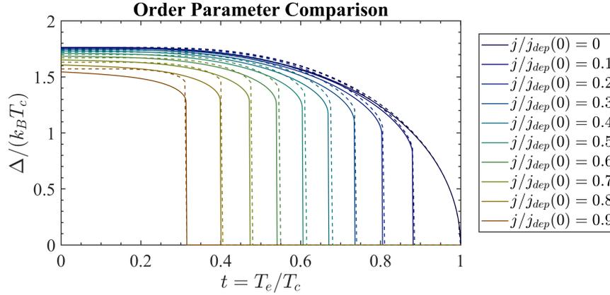
Figure 3.9: Comparison of the stationary state order parameter at various bias currents within the Vodolazov TDGL model (solid lines) and Usadel model (dashed lines). The vertical discontinuities correspond to the temperature where the current exceeds the critical depairing current.
