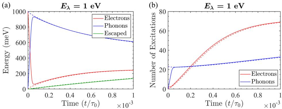
Figure 2.12: Comparison of downconversion calculations using the electron bubble (solid lines) and phonon plateau (dashed lines) initial conditions with strong electron-electron interactions where  $\alpha_{e-e} = 500$ . The energy partitioning is shown in (a) while the average number of excitations is shown in (b). There is minimal difference between the two results.
