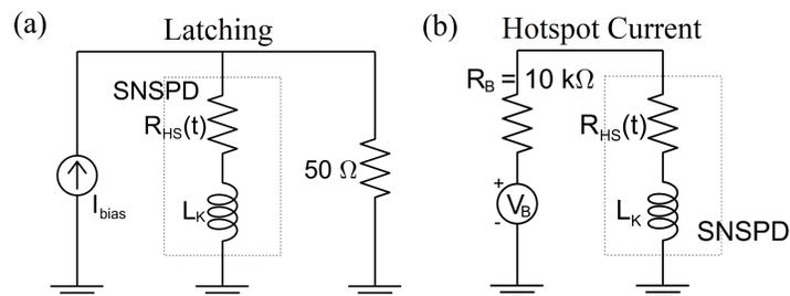
Figure 4.11: Circuit equations used for modeling (a) latching and (b) hotspot current behavior. A capacitor could be added to the output between the SNSPD and  $50\ \Omega$  termination of the latching circuit to better represent the presence of a bias-tee, but for the reset time constants probed in this work, the capacitance of a typical bias-tee does not influence the dynamics.
