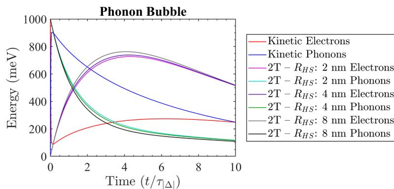
Figure 3.27: Comparison of the kinetic downconversion model with the two-temperature model in the case of cylindrical expansion of a hotspot using the modified phonon bubble initial conditions. Changes to the hotspot size of the modified phonon bubble do not strongly influence the energy evolution and partitioning of the system.
