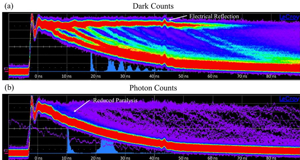
Figure 4.16: Paralysis in the WSi detector with an electrical recovery time constant of 27.2 ns for (a) dark counts (b) photon counts when biased at  $8.6 \mu\text{A}$  at a bath temperature of 875 mK. The paralysis effect is much more pronounced for dark counts compared to photon counts.
