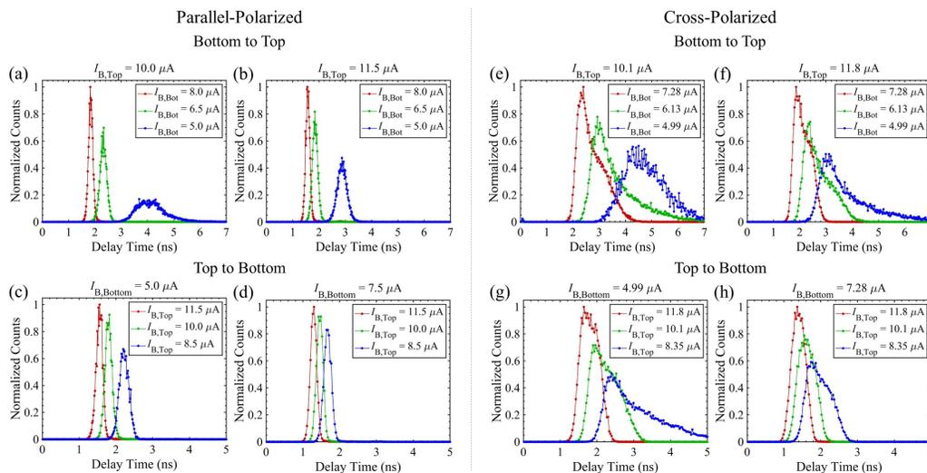
Figure 5.6: Thermal coupling delay histograms for parallel-polarized (a-d) and cross-polarized devices (e-h). The coupling efficiency increases as both the source and receiving channel bias currents increase. Coupling from the bottom to top layer is less efficient than top to bottom due to the lower overall bias current and lower Joule heat generated during a detection.
