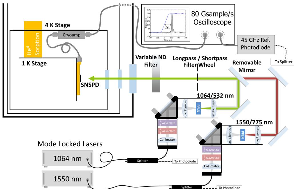
Figure 3.2: Low jitter experimental setup. Two mode-locked lasers (1550 nm and 1064 nm) are focused into second harmonic generation crystals to produce 775 nm and 532 nm light. After a wavelength is selected by appropriate use of a longpass or shortpass filter, light is free space coupled into the cryostat and onto the detector. The signal from the SNSPD is amplified using a cryogenic amplifier operating at 4 K before being recorded by a 80 gigasample per second oscilloscope.
