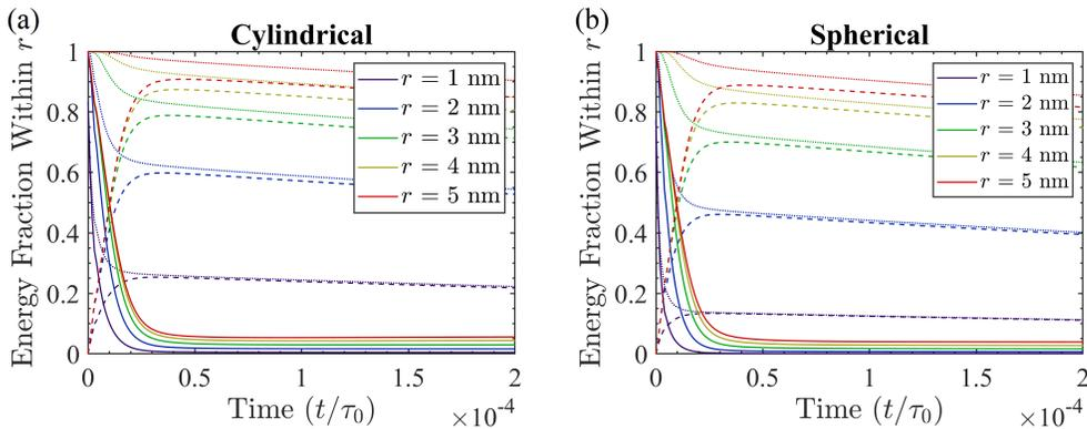
Figure 2.8: Fraction of energy within a given radius as a function of time for (a) cylindrical and (b) spherical coordinates. The solid line shows the electron system, the dashed line is the phonon system, and the dotted line is the combined system. The majority of the energy remains localized to within a few nanometers of the absorption location due to phonon localization.
