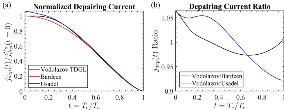
Figure 3.8: Comparison of the stationary current-carrying state within the Vodolazov TDGL model to the solution of the Usadel equations and Bardeen equation. The temperature-dependent depairing current (a) shows good agreement between all three models for  $T_e > T_c/2$ . The largest error in the ratio of Vodolazov's model to the other two (b) remains below 7% over the entire temperature range.
