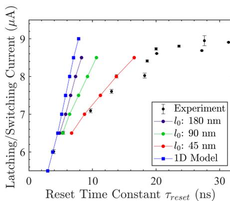
Figure 4.21: Comparison of latching in experiment and using the 3D three-temperature electrothermal model. Fitting to experiment can only be achieved by assuming a phonon mean free path  $l_0$  four times smaller than that extracted from the nanowire thermometry measurements. The result of the 1D model with the same WSi material parameters is shown for comparison.
