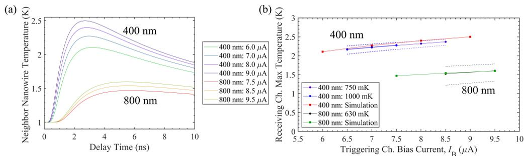
Figure 4.22: (a) Temperature rise in an adjacent nanowire for simulated detections in the 400 nm and 800 nm pitch devices. The timescale of the temperature rise is faster than observed experimentally for the 400 nm pitch device. (b) Comparison of maximum temperature reached in adjacent nanowires for simulation and experiment. There is reasonable agreement between the model and experiment.
