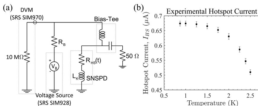
Figure 4.4: (a) Experimental setup for hotspot current and latching measurements. (b) Hotspot current vs bath temperature experimental results.
