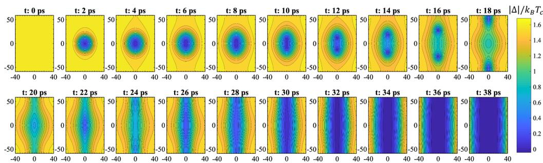
Figure 3.10: Evolution of the magnitude of the order parameter for a detection in the center of a 120 nm wire. The vertical scale is the transverse coordinate  $y$  while the horizontal scale is the longitudinal coordinate  $x$  with the bias current flowing from left to right. The formation of a vortex/antivortex pair and subsequent motion of the pair to the edge of the nanowire facilitates the suppression of superconductivity.
