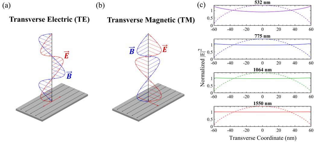
Figure 3.4: Orientation of the (a) TE and (b) TM polarizations with respect to the nanowire. (c) Electric field profile in a 120 nm NbN nanowire encapsulated in SiO<sub>2</sub> for the four wavelengths of interest for experimental measurements. Solid lines indicate the TE mode while dashed lines are the TM mode. Calculations were performed using FDTD software on a CPW structure with the same dimensions as the experimental devices.
