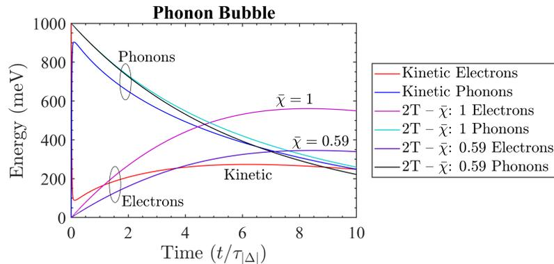
Figure 3.29: Comparison of the kinetic downconversion model with the two-temperature model for the case of cylindrical expansion of a hotspot using the modified phonon bubble initial conditions with  $\tau_{DC}$  increased by a factor of 4.
