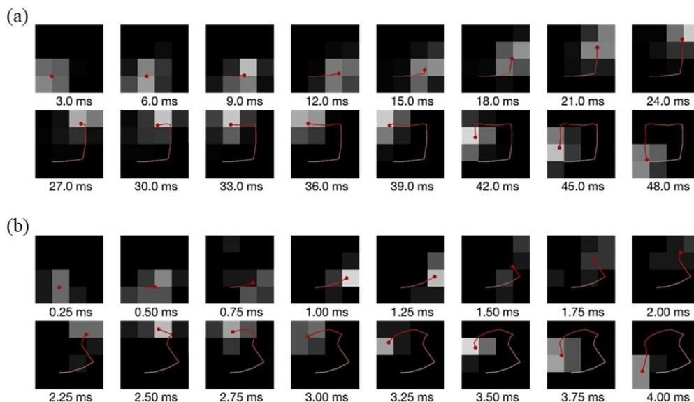
Figure 5.10: Laser spot tracking in a square pattern using the cross-polarized array. (a) Tracking using a 48 ms period and 3 ms frames with an average of 146.5 photon detections per frame. (b) Tracking using a 4 ms period and 250  $\mu$ s frames with an average of 11.7 photon detections per frame. The red circle indicates the centroid of the detections for a given frame and the line shows the path of the centroid for the sequence of frames.
