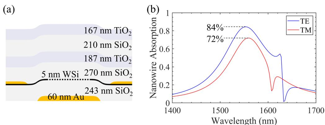
Figure 6.2: (a) Cross-section of the detector. The design consists of two bi-layers of  $\text{SiO}_2$  and  $\text{TiO}_2$  forming the AR coating and a Au mirror forming the back reflector. (b) Model of the optical absorption in the nanowire layer calculated using RCWA software.
