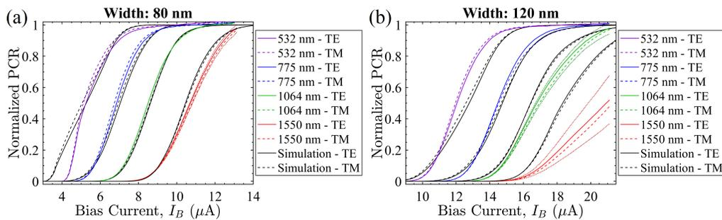
Figure 3.26: Fitting of the model to experiment for (a) 80 nm width and (b) 120 nm width devices while using  $\tau_{DC}$  increased by a factor of 4 compared to the average value for phonons of the phonon plateau.
