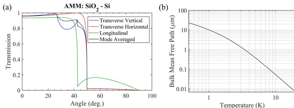
Figure 4.19: (a) AMM predictions of the phonon transmission for an  $\text{SiO}_2$  - Si interface. (b) Bulk phonon mean free path for  $\text{SiO}_2$ .
