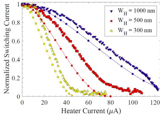
Figure 4.27: Normalized switching current of hTrons (symbols) with heater widths of 300 nm, 500 nm, and 1000 nm as a function of the heater current. The channel width is kept at 200 nm for these devices. Predictions from the electrothermal model (lines) are shown for comparison.
