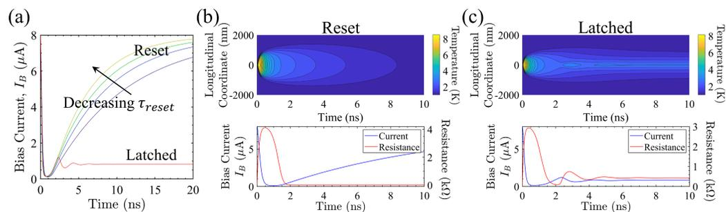
Figure 4.2: (a) Emergence of latching as the electrical reset time  $\tau_{reset}$  decreases. In the case of (b) proper recovery the resistance of the device returns to zero after a detection and the temperature (shown in top) relaxes back to the substrate temperature. In contrast, for a (c) latching device, the resistance remains finite, and a segment of the nanowire remains at a temperature above  $T_c$ .
