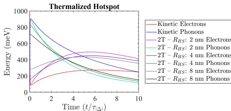
Figure 3.28: Comparison of the kinetic downconversion model with the two-temperature model in the case of cylindrical expansion of a hotspot using the modified phonon bubble initial conditions.
