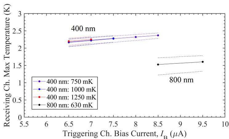
Figure 4.10: Estimated maximum temperature reached during crosstalk. The top group of curves shows the 400 nm pitch data for the three bath temperatures measured while the low curve show the 800 nm pitch data at 630 mK. The dashed lines show the approximate uncertainty bounds of the calculation.
