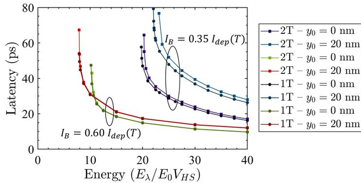
Figure 3.30: Comparison of the latency calculations for the one-temperature (dark circles) and two-temperature (squares) models for the energy balance within the TDGL equations. There is only a small difference between the two results. The material parameters are the same as throughout with  $\gamma = 20$ ,  $\tau_{esc} = 9.4$  ps, and  $\tau_{ee}(T_c) = 5$  ps.
