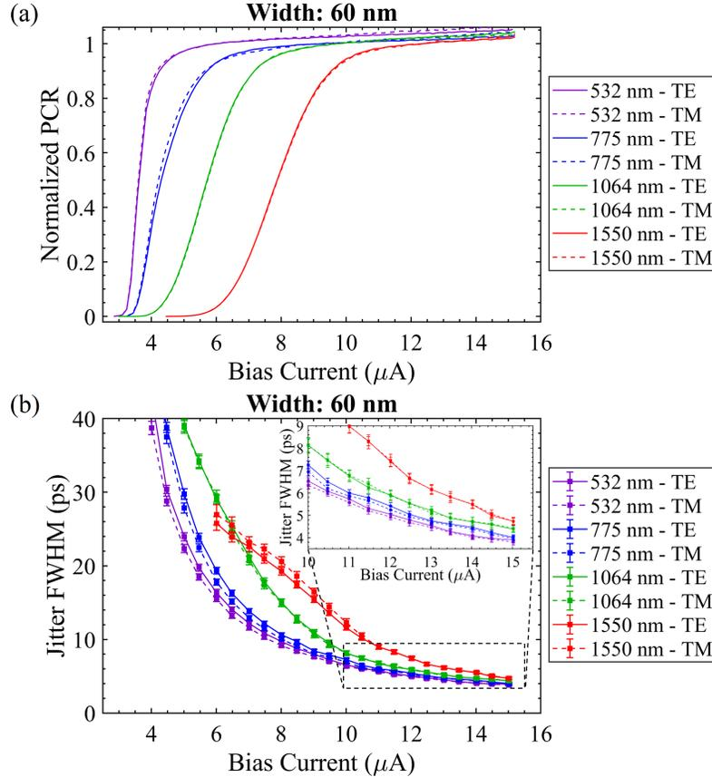
Figure 3.6: Polarization-dependent (a) PCR and (b) timing jitter for a 60 nm NbN device measured at a bath temperature of 1 K. Solid lines indicate the TE polarization and dashed lines show the TM polarization.
