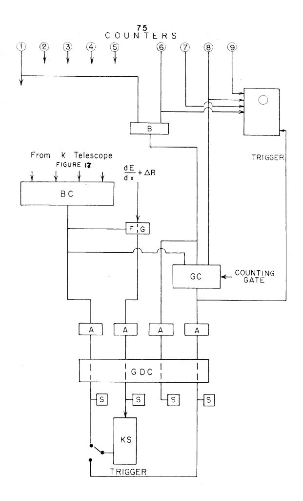
For this experiment, the bias coincidence circuit also opened the fast gate which passed the  $dE/dx + \Delta R$  pulse.
