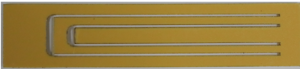
Figure E.5 – A laser cut plastic shim with double-sided adhesive tape
