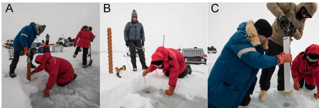
Figure D.2 – Ice coring in Utqiagvik (formerly Barrow), Alaska. (A) The interrupted coring technique is used to drill into sea ice, while another team member clears ice chips from the drill site. A third team member has completed the process of clearing the snow cover from the planned coring area. (B) Using a weighted depth gauge to measure the sea ice thickness through a borehole drilled through the ice to underlying seawater; the gauge is designed to anchor to the underside of the ice for a taught pull upwards. (C) Using core retrieval tongs to pull a partial ice core out of the sea ice cover and establish a “sackhole” for the accumulation of sea ice brine. Photos courtesy of Anders Torstensson.
