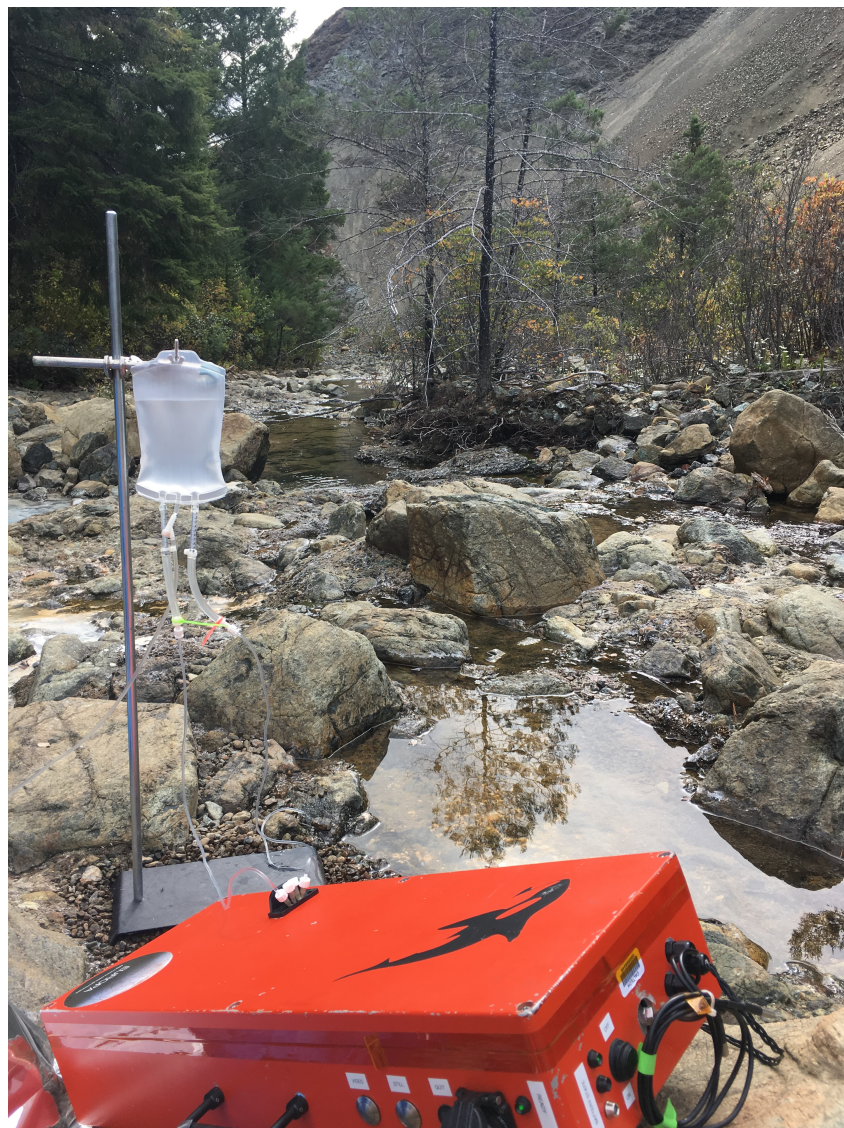
Figure C.2 – Experimental setup of the in-field pulsation dampener
