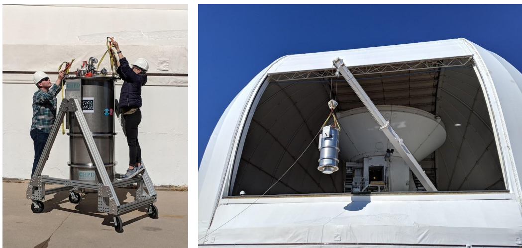
Figure 6.1: Photos from the installation of the TIME receiver on the 12 meter ALMA prototype antenna at Kitt Peak in southern Arizona.
