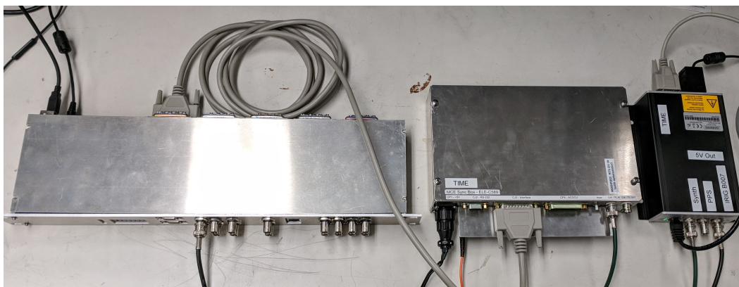
Figure 2.25: The key timing boxes used in TIME. Left to right: HKMBv1 housekeeping readout box, MCE Sync Box, Meinberg SyncBox/N2X
