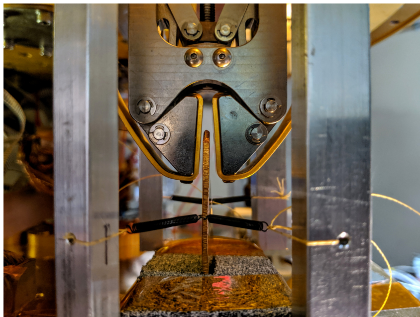
Figure 2.5: One of two mechanical heat switches connecting the 4K stage to the focal plane during the cool-down process. Heat switches from High Precision Devices. Heat strap suspension system by Yun-Ting Cheng.
