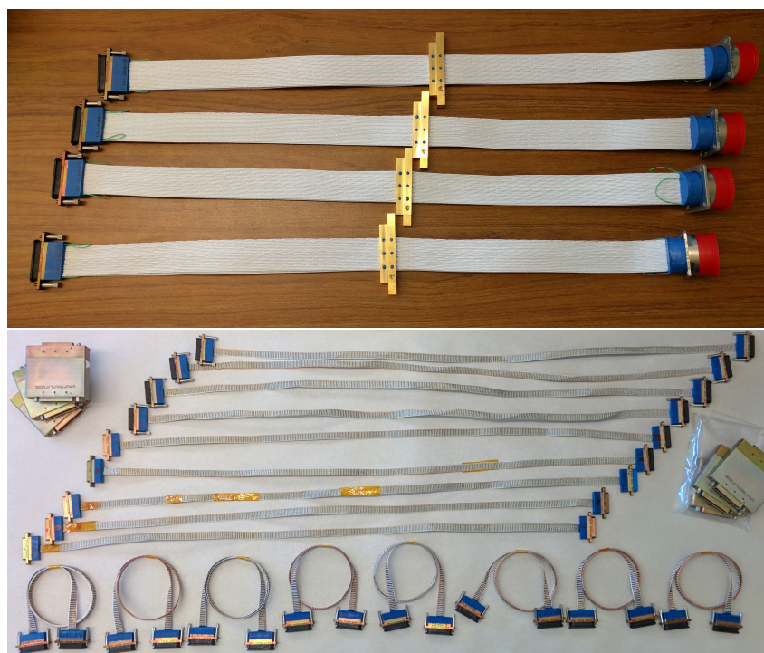
Figure 2.19: Upper: Four of the ten 100 pin Manganin detector cables running from the 300K vacuum flange to the 4K electronics box. Lower: A set of 37 pin superconducting NbTi cables joining the 4K electronics box to the UC distribution board.
