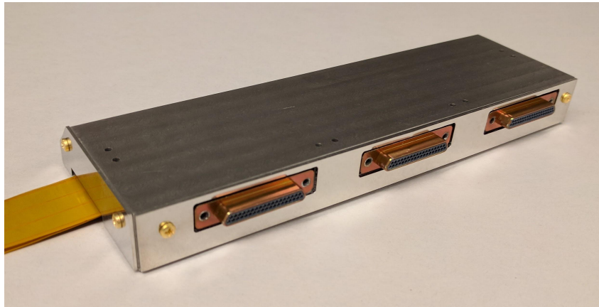
Figure 2.29: Top : An exploded render of a TIME SQUID board housing. Superconducting material (Al) is shown in yellow and high- \mu metal (A4K) is shown in magenta. Bottom : One of 12 TIME SQUID boards. Reprinted by permission from Springer Nature: Hunacek et al. J Low Temp Phys [50], © 2018
