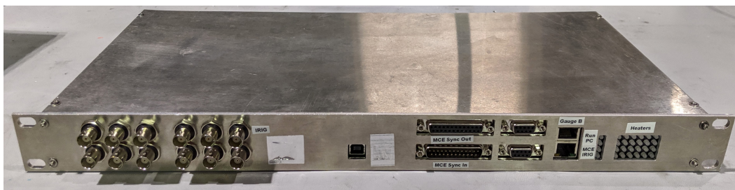
Figure C.10: The TIME HKMBv2 box in its rack-mount enclosure. Connectors for the thermometry and heaters are found on the reverse side.
