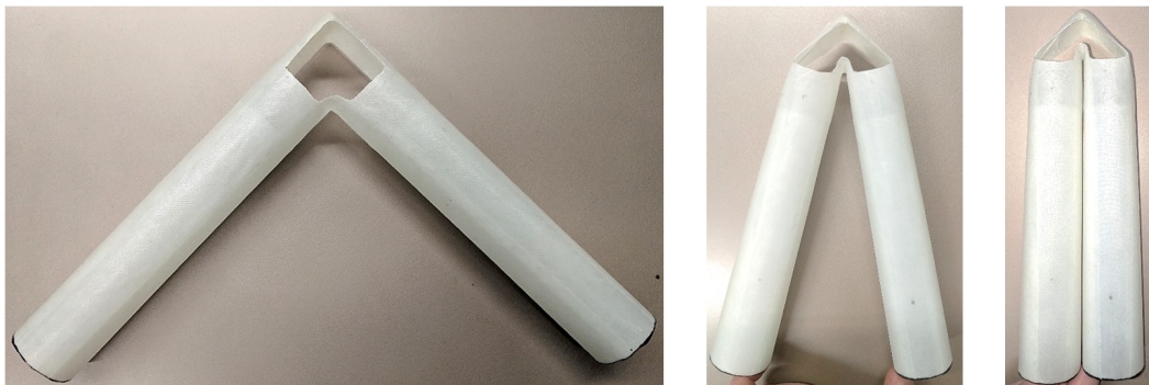
Figure A.3: Example of thin shell built using the silicone molding manufacturing technique.
