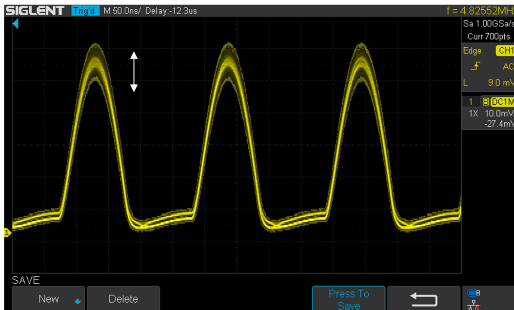
Figure 4.6: The time domain oscillation voltage waveform measured across one of the coil terminals and ground. The amplitude noise resulted from the current injection is indicated by the white double arrow.
