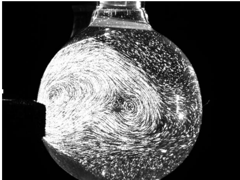
Figure 3.7: Pathline visualization from 5-celsius temperature difference (center heating) These 100 images were taken from 5 mins to 5 mins and 10 secs. Note that most of the flow behavior was happening on the left half of the eye model.
