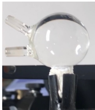
(a) Actual picture of an eye model with openings for injection
