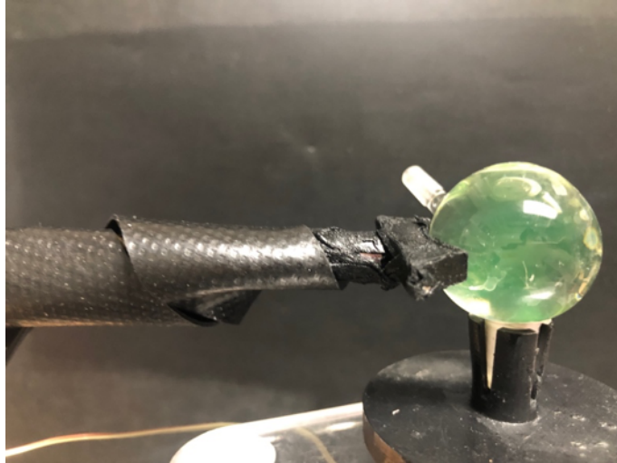
Figure 3.4: Heating element at the “center” heating location
