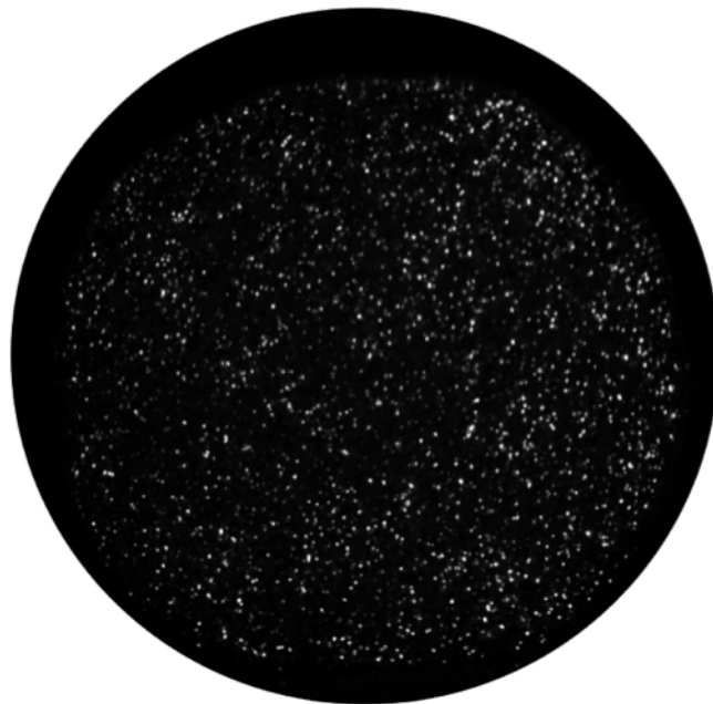
Figure 2.10: Example of an image captured during a PIV visualization session
