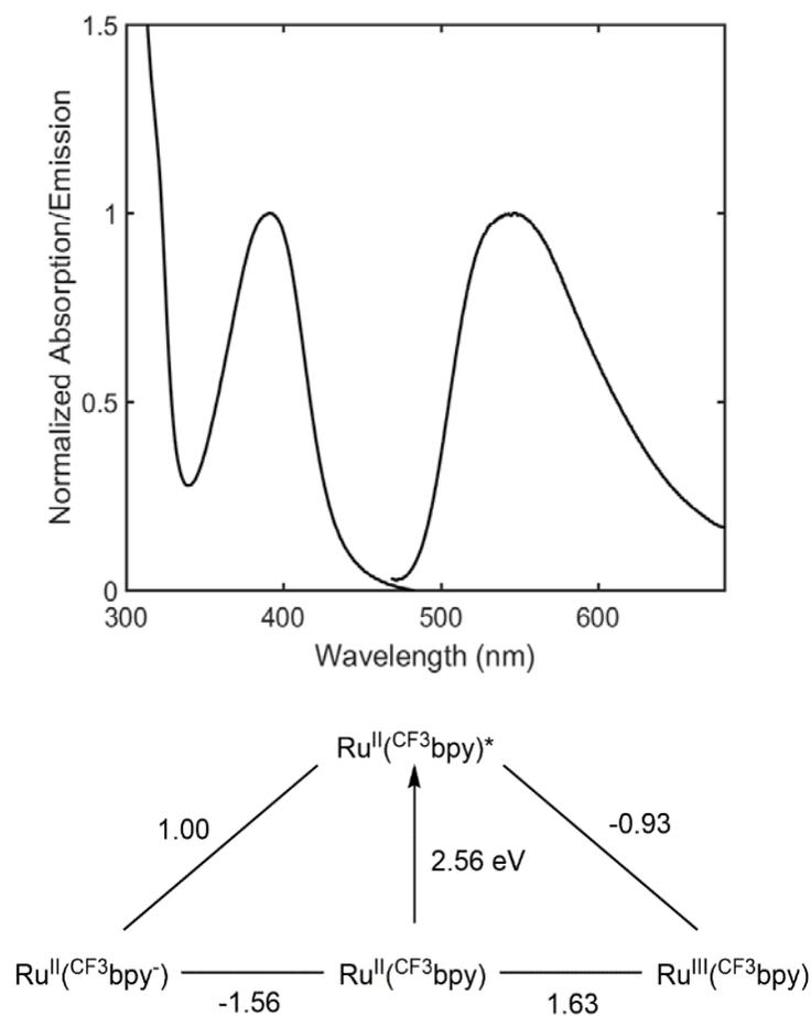
**Figure 10:** Top: room temperature absorption and emission data for  $[\text{Ru}(\text{CF}_3\text{bpy})(\text{CN-BCF})_4]^{2-}$  in acetonitrile. Bottom: Modified Latimer diagram with potentials given in V vs.  $\text{Fc}^{+/0}$ .
