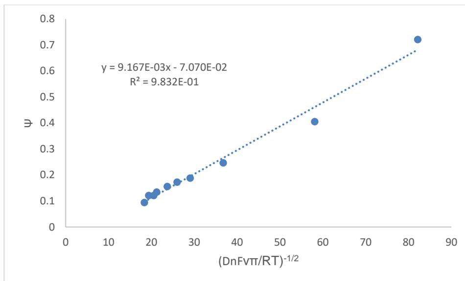
**Figure S5:** Nicholson analysis of the  $^{CF_3}bpy^{0/-}$  couple of  $PPN_2Ru(^{CF_3}bpy)(CN-BCF)_4$ , with a slope of  $k_0$ .
