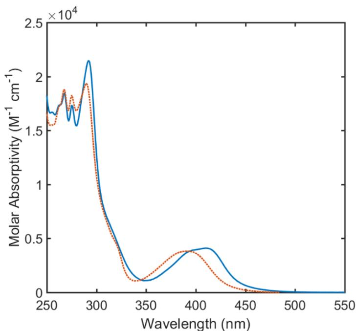
**Figure 8:** UV-Vis spectra for  $\text{PPN}_2\text{Ru}(\text{CF}_3\text{bpy})(\text{CN-BCF})_4$  in DCM (blue solid trace) and MeCN (orange broken trace).
