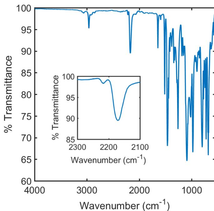
**Figure 7:** IR spectrum of PPN<sub>2</sub>Ru(CF<sub>3</sub>bpy)(CN-BCF)<sub>4</sub> with CN stretches highlighted in inset.
