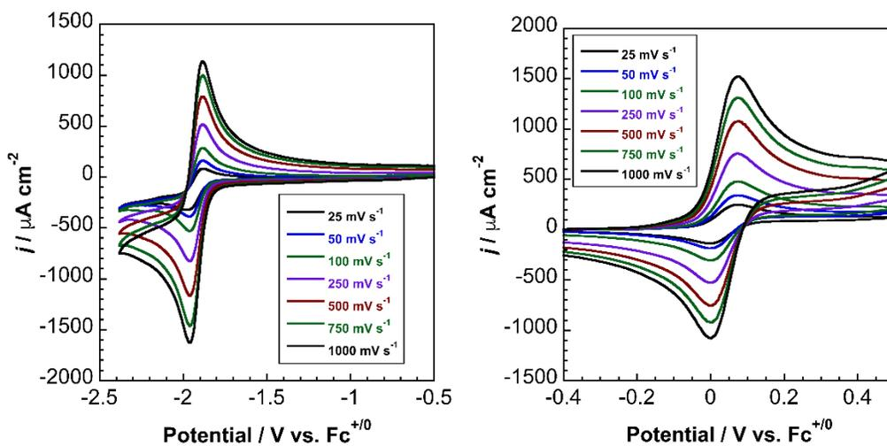
**Figure S2:** Variable scan rate cyclic voltammograms for  $\text{PPN}_2\text{Ru}(\text{CF}_3\text{bpy})(\text{CN})_4$ . 33 mM  $\text{PPN}_2\text{Ru}(\text{CF}_3\text{bpy})(\text{CN})_4$  in 0.2 M  $\text{Bu}_4\text{NPF}_6$ -supported acetonitrile. Working electrode: glassy carbon. Counter electrode: Pt wire.
