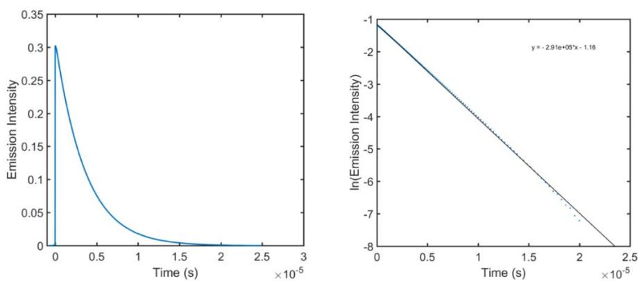
**Figure S7:** Left, time-resolved luminescence data for  $\text{PPN}_2\text{Ru}(\text{CF}_3\text{bpy})(\text{CN-BCF})_4$ . Right, linear fit to determine lifetime. The slope of the fit is the inverse of  $\tau = 3.44 \mu\text{s}$ .
