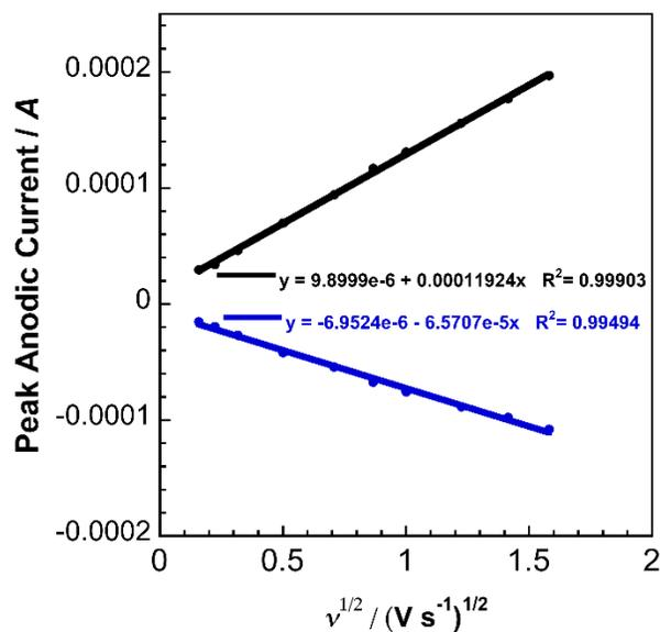
**Figure S3:** Randles-Sevcik plot for  $\text{PPN}_2\text{Ru}(\text{CF}_3\text{bpy})(\text{CN-BCF})_4$ ;  $D = 7.4 \times 10^{-6} \text{ cm}^2 \text{ s}^{-1}$  (top),  $2.4 \times 10^{-6} \text{ cm}^2 \text{ s}^{-1}$  (bottom).
