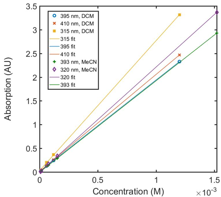
**Figure S9:** Dilution series for molar absorptivity of  $\text{PPN}_2\text{Ru}(\text{CF}_3\text{bpy})(\text{CN-BCF})_4$  and linear fits. All measurements in 5 mm cuvette. Extinction coefficients are  $\epsilon_{315} = 1460 \text{ M}^{-1}\text{cm}^{-1}$ ,  $\epsilon_{395} = 958 \text{ M}^{-1}\text{cm}^{-1}$ ,  $\epsilon_{410} = 1020 \text{ M}^{-1}\text{cm}^{-1}$  in DCM and  $\epsilon_{320} = 3860 \text{ M}^{-1}\text{cm}^{-1}$ ,  $\epsilon_{393} = 4440 \text{ M}^{-1}\text{cm}^{-1}$  in MeCN.
