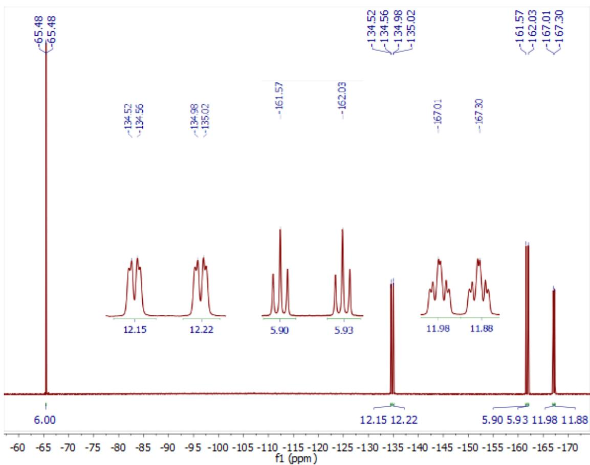
**Figure S13:**  $^{19}\text{F}$  NMR spectrum of  $\text{PPN}_2\text{Ru}(\text{CF}_3\text{bpy})(\text{CN-BCF})_4$  in  $\text{CD}_2\text{Cl}_2$  with insets showing detail of BCF peaks.
