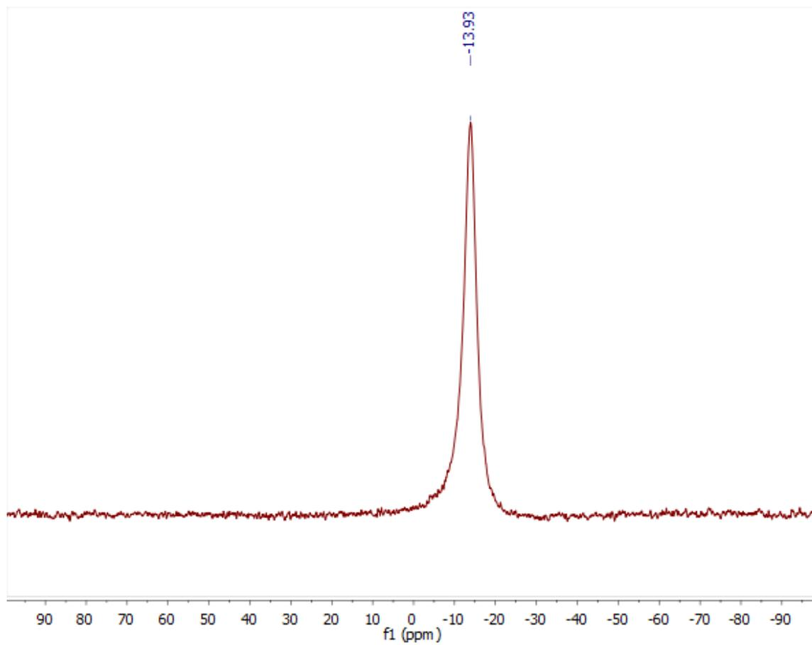
**Figure S12:**  $^{11}\text{B}$  NMR spectrum of  $\text{PPN}_2\text{Ru}(\text{CF}_3\text{bpy})(\text{CN-BCF})_4$  in  $\text{CD}_2\text{Cl}_2$  acquired in a quartz NMR tube.
