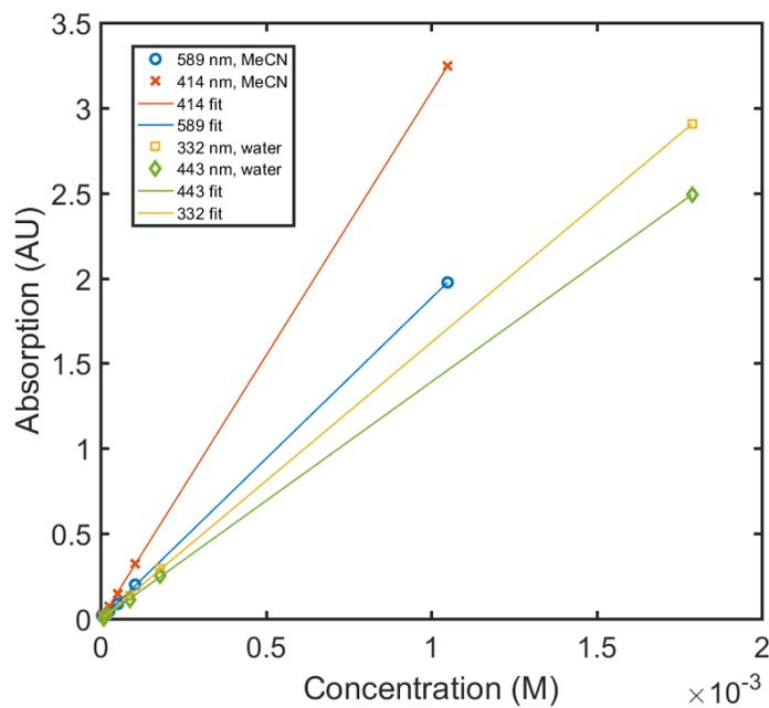
**Figure S8:** Dilution series for molar absorptivity of  $[\text{Ru}(\text{CF}_3\text{bpy})(\text{CN})_4]^{2-}$  (K salt in water, PPN salt in MeCN) and linear fits. All measurements in 5 mm cuvette. Extinction coefficients are  $\epsilon_{332} = 3660 \text{ M}^{-1}\text{cm}^{-1}$ ,  $\epsilon_{443} = 3170 \text{ M}^{-1}\text{cm}^{-1}$  in water and  $\epsilon_{414} = 6190 \text{ M}^{-1}\text{cm}^{-1}$ ,  $\epsilon_{589} = 3770 \text{ M}^{-1}\text{cm}^{-1}$  in MeCN.
