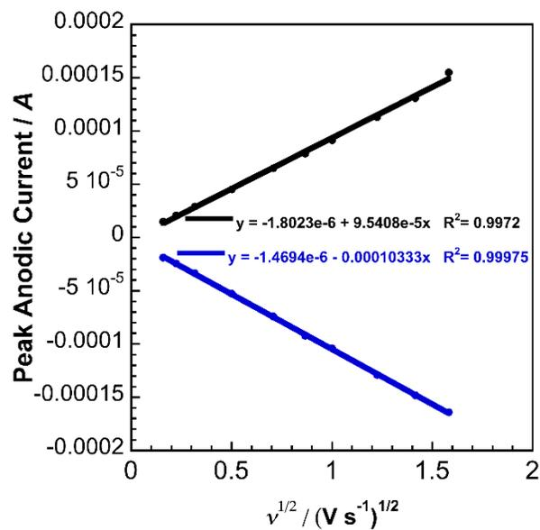
**Figure S1:** Randles-Sevcik plot for  $\text{PPN}_2\text{Ru}(\text{CF}_3\text{bpy})(\text{CN})_4$ ;  $D = 5.7 \times 10^{-6} \text{ cm}^2 \text{ s}^{-1}$ .
