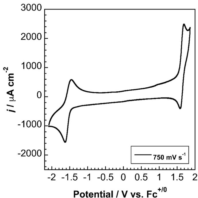
**Figure 9:** Cyclic voltammogram of 2.3 mM  $\text{PPN}_2\text{Ru}(\text{CF}_3\text{bpy})(\text{CN-BCF})_4$  in 0.2 M  $\text{Bu}_4\text{NPF}_6$ -supported acetonitrile. Working electrode: glassy carbon. Counter electrode: Pt wire.
