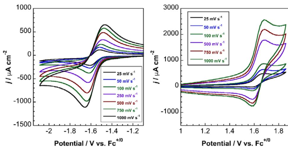
**Figure S4:** Variable scan rate cyclic voltammetry of  $\text{PPN}_2\text{Ru}(\text{CF}_3\text{bpy})(\text{CN-BCF})_4$ . . 2.3 mM  $\text{PPN}_2\text{Ru}(\text{CF}_3\text{bpy})(\text{CN-BCF})_4$  in 0.2 M  $\text{Bu}_4\text{NPF}_6$ -supported acetonitrile. Working electrode: glassy carbon. Counter electrode: Pt wire.
