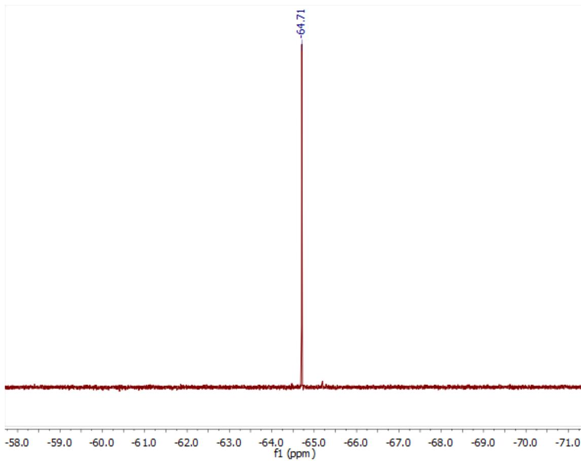
**Figure S10:**  $^{19}\text{F}$  NMR spectrum of  $\text{PPN}_2\text{Ru}(\text{CF}_3\text{bpy})(\text{CN})_4$  in  $\text{CD}_2\text{Cl}_2$ .
