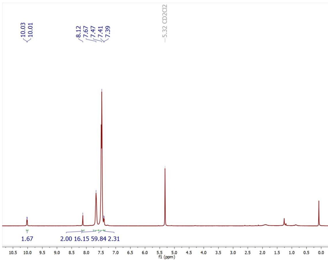
**Figure S11:**  $^1\text{H}$  NMR spectrum of  $\text{PPN}_2\text{Ru}(\text{CF}_3\text{bpy})(\text{CN})_4$  in  $\text{CD}_2\text{Cl}_2$ . Peaks upfield of 3 ppm are attributable to water, trace solvents, and silicone grease.
