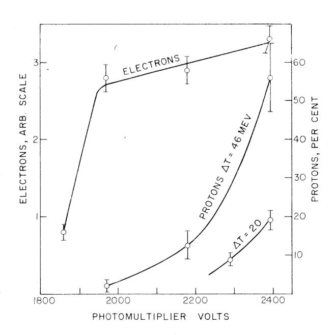
peaks there were easier to separate than in counter 1. The bias settings had to be checked at frequent intervals since they and the photomultiplier gains drifted slightly from time to time.
