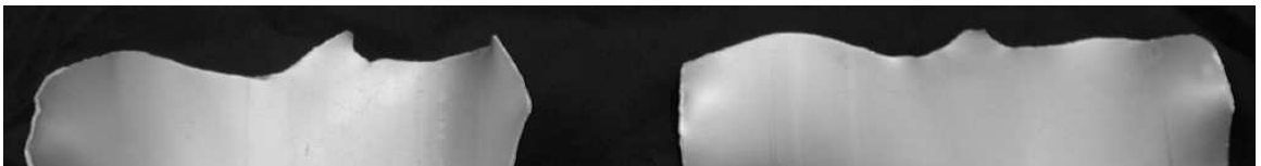
Figure 4.13: Resemblance of the forward bifurcated crack paths of two L = 50.8 mm notch specimens. The repeated experiments were run to demonstrate reproducibility (Shot 7 on the left and Shot 6 on the right).
