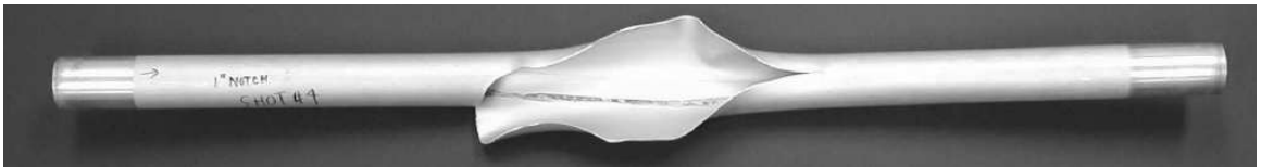
Figure 4.10: Ruptured tube with initial L = 25.4 mm notch (Shot 4).
