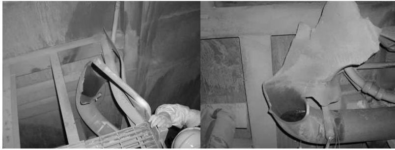
Figure 1.2: Two ends of a ruptured section of a steam pipe from the Hamaoka Nuclear Power Plant accident (2001).
