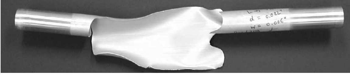
Figure 4.19: Shot 24 specimen. Detonation wave ran from left to right.
