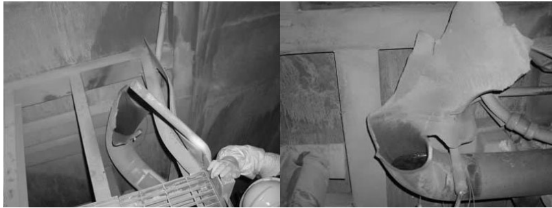
Figure 1.2: Two ends of a ruptured section of a steam pipe from the Hamaoka Nuclear Power Plant accident (2001).
