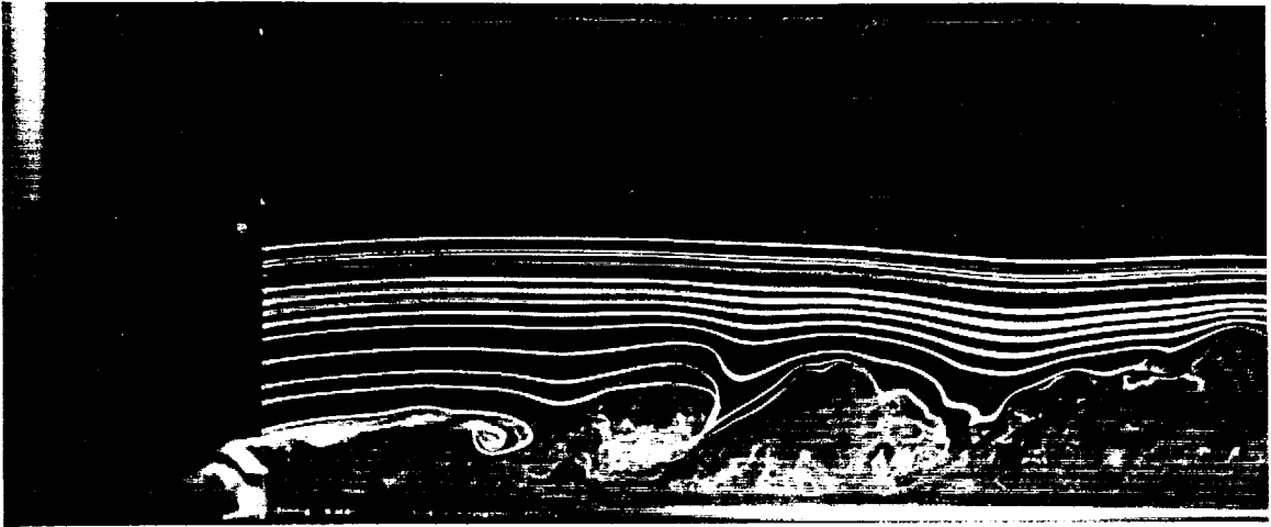
FIG. 5.11 Smoke wire flow visualization of shear layer vortices, \sigma = 0.65 , Re = 2600
