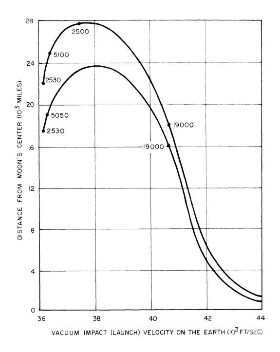
[NUMBERS ON GRAPH INDICATE ACTUAL VELOCITY OF VEHICLE AT GIVEN DISTANCE (FT/SEC)]
