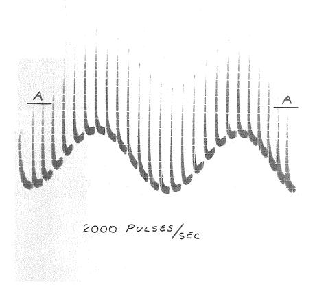
FIG. 4: DIFFERENTIAL AMPLIFIER OUTPUT FOR A SINE WAVE INPUT
