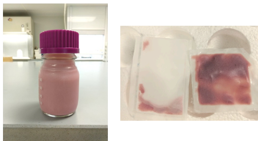
Figure 4.7: CA-CPG beads dispersed in 50 mM pH 7 phosphate buffer (left) and sealed within 70 \mu\text{m} mesh bags (right)
