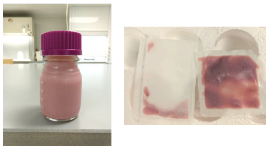
Figure 4.7: CA-CPG beads dispersed in 50 mM pH 7 phosphate buffer (left) and sealed within 70 \mu m mesh bags (right)
