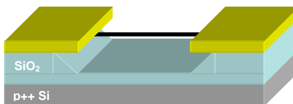
Figure II-4. Schematic diagram of metal electrodes as the etch mask. Undercut structures are always present after etching.
