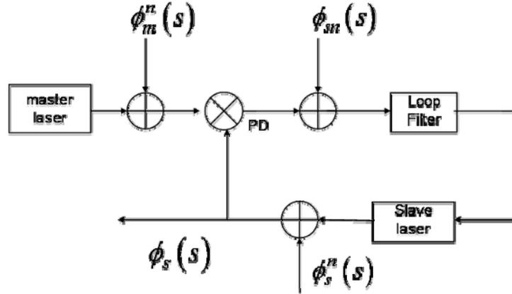
Fig. 2.4 Sources of phase noise in an OPLL
