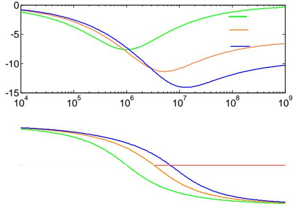
Fig. 2.8 FM response of single-section DFB lasers calculated with the modified low-pass filter model. The fitting parameters are:  $f_c = 1\text{MHz}$  and  $b = 1, 2$  and  $3$ .
