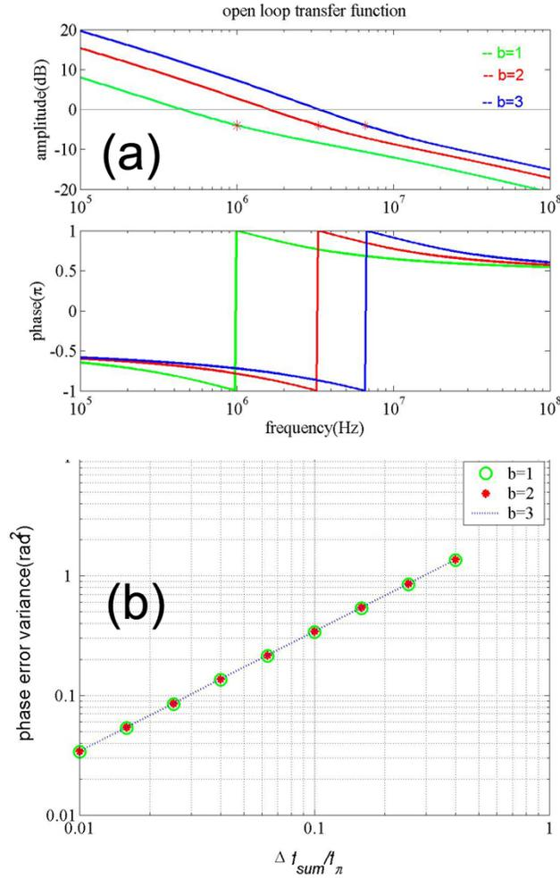
Fig. 2.9 (a) The Bode plots of the open loop transfer functions for different values of the fitting parameter  $b$  in Eq. (2.34). (b) The variance of the differential phase error as a function of the normalized laser linewidth  $\Delta f / f_{\pi}$ .
