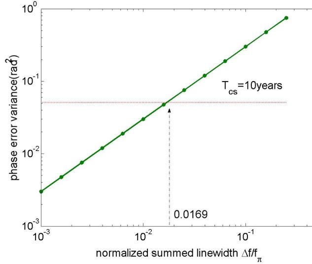
Fig. 2.7 The variance of the differential phase error as a function of the normalized summed laser linewidth  $\Delta f / f_\pi$ .  $f_\pi = 1/4\tau_d$  is the  $\pi$  phase lag frequency given by the loop delay.  $T_{cs}$  is the average time between cycle slips defined in Eq. (2.25).
