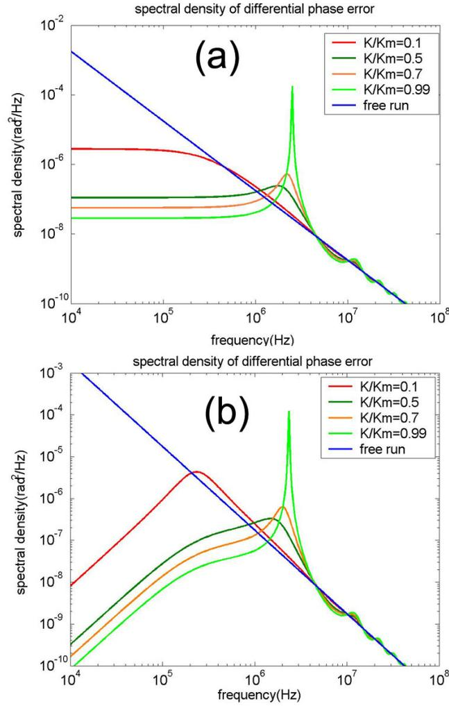
Fig. 2.5 The spectral density functions of the differential phase error  $\phi_e$  for different small signal loop gain  $K$ .  $K_m$  is the maximum allowable loop gain determined by the stability criterion. (a) No loop filter is used. (b) An active second-order filter  $(1 + f/f_0)/(f/f_0)$  is used. In both (a) and (b), a loop delay of 100 ns is assumed.
