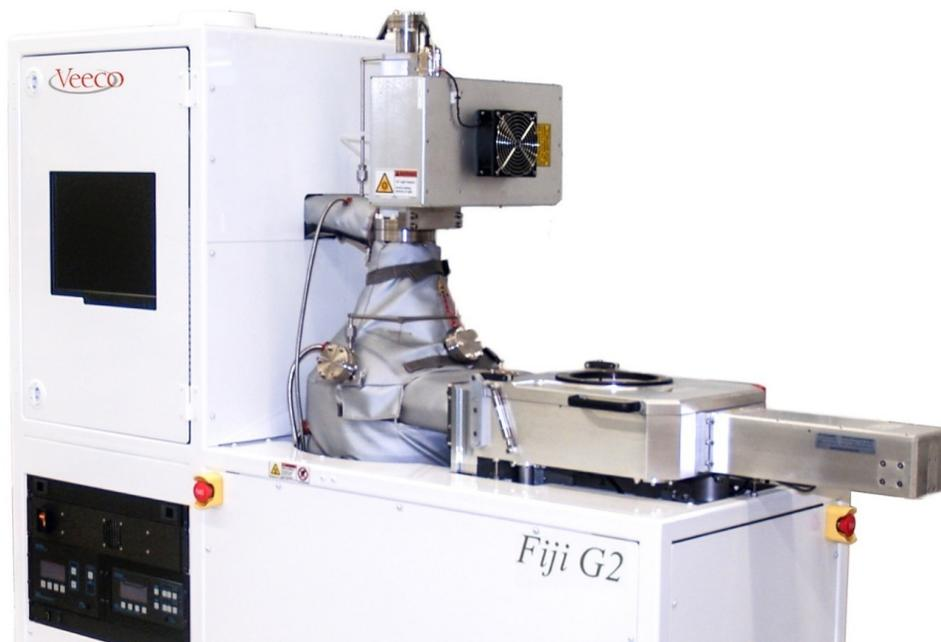
Figure 7.6: The Atomic Layer Deposition (ALD) tool we used. The plasma tube is later upgrade with a metal Hollow Cathode Plasma (HCP) tube to eliminate Oxygen contamination due to deteriorating quartz ICP plasma tube.
