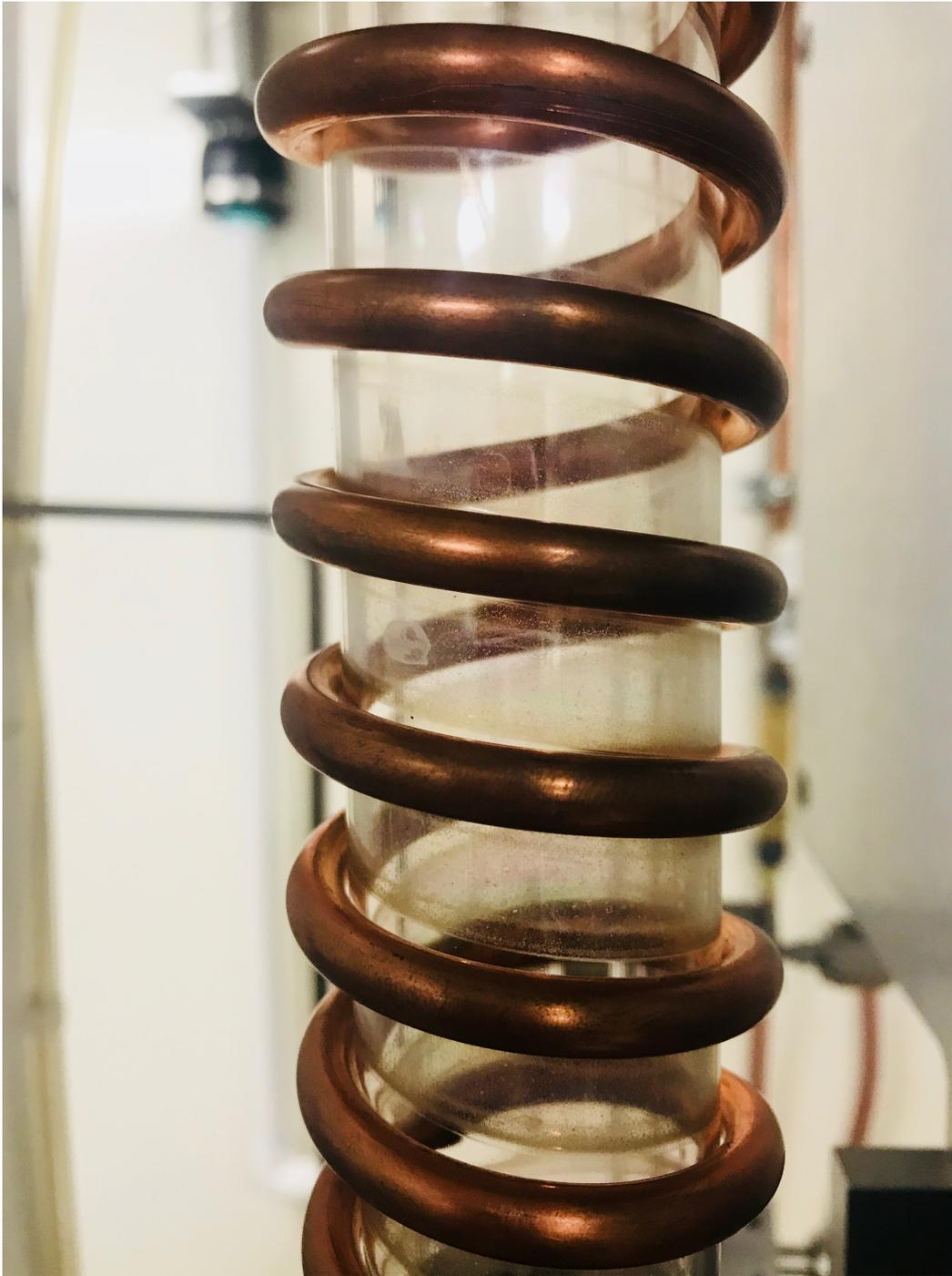
Figure 7.10: The burned quartz plasma tube that was etched by the high power plasma and generated excessive Oxygen into the ALD process chamber and contaminated the ultra Oxygen sensitive AlN process and caused deteriorating chamber condition that yielded inconsistent AlN deposition results.
