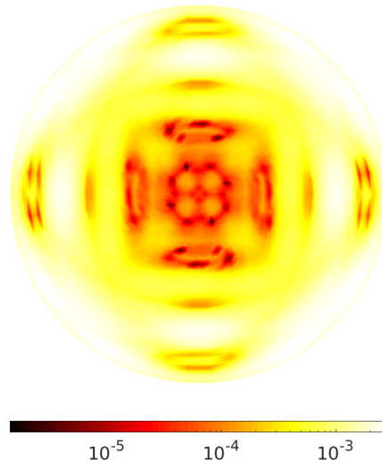
Figure 5.10: Energy balance error for a periodic crossed-grating with period equal to 5\lambda as a function of the incidence direction. The unit-cell of the grating is divided in four non-overlapping patches (obtained from a single dyadic splitting of the parameter square [-1, 1]^2 and a re-scaling of the parameters) and each is discretized with 16 \times 16 Chebyshev grid points. The evaluation of the quasi-periodic Green function is performed by means of Ewald method truncating each of the required series with \|m\|_\infty < 20 ; see also Remark 4.
