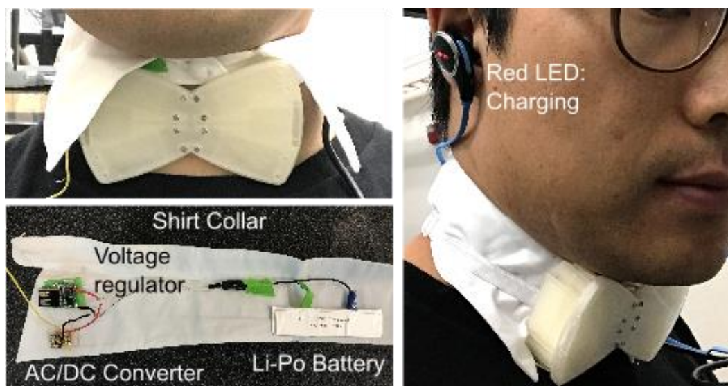
Figure 5.16: Bow tie shaped energy harvester using a 4-energy harvesting array. The battery and circuits were placed inside the shirt collar to charge the Bluetooth headphones.
