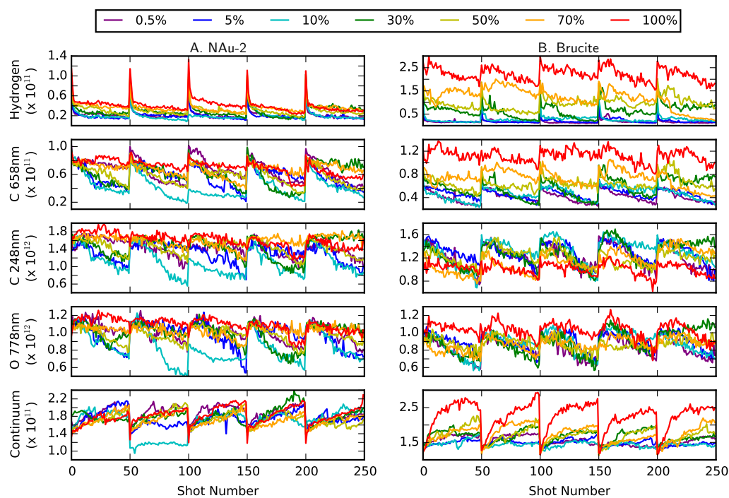
Figure 6. Variation in H, C (II) 658-nm, C (I) 656-nm, and O (I) 778-nm peak areas and continuum emission nearby H (660 nm) with shot number for a low-moderate weight percent H mixture (NAu-2) and a high weight percent H mixture (brucite). Each 50 shots is a different location on the sample and colors indicate increasing weight percent NAu-2 or brucite.
