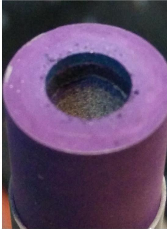
Figure 2.8: Detail of the contaminant deposited on the inside of the insert.
