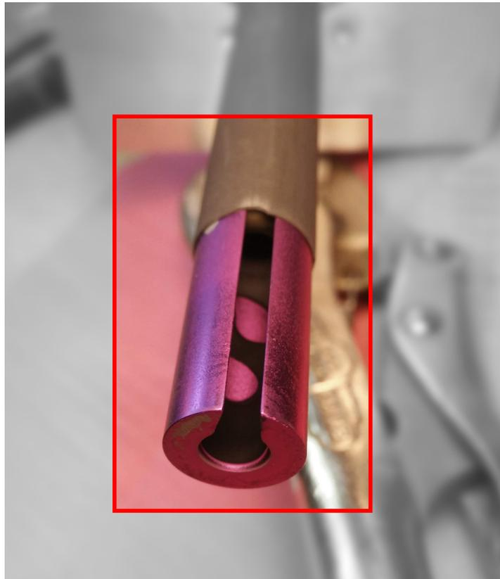
Figure 4.10: Test sample (part B) after the 50 hr test. Sample shows carbon contamination in most of its internal area.
