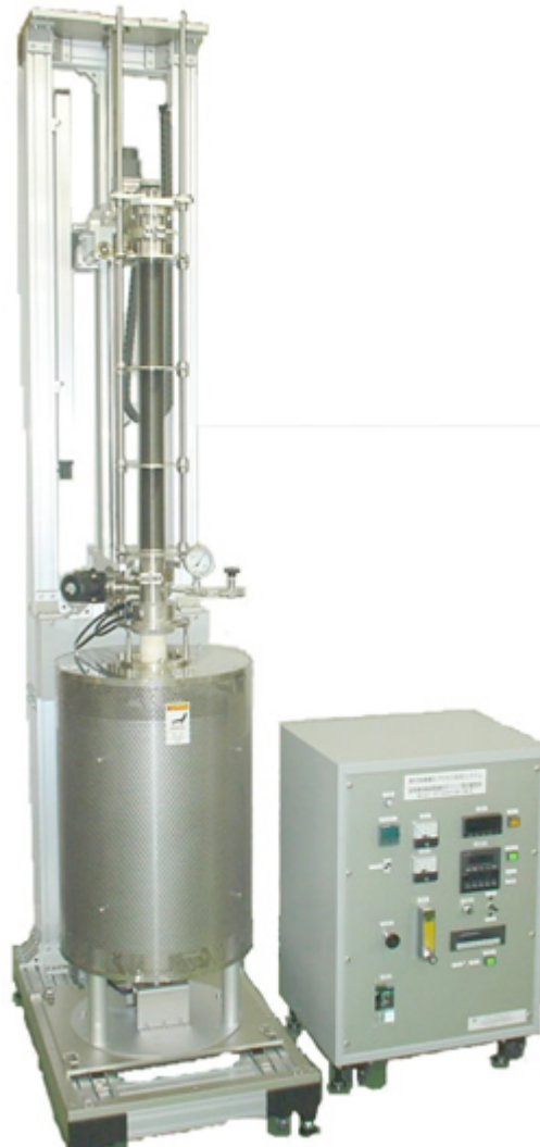
Figure B.6 The Bridgeman vertical tube furnace and crane assembly (218).
