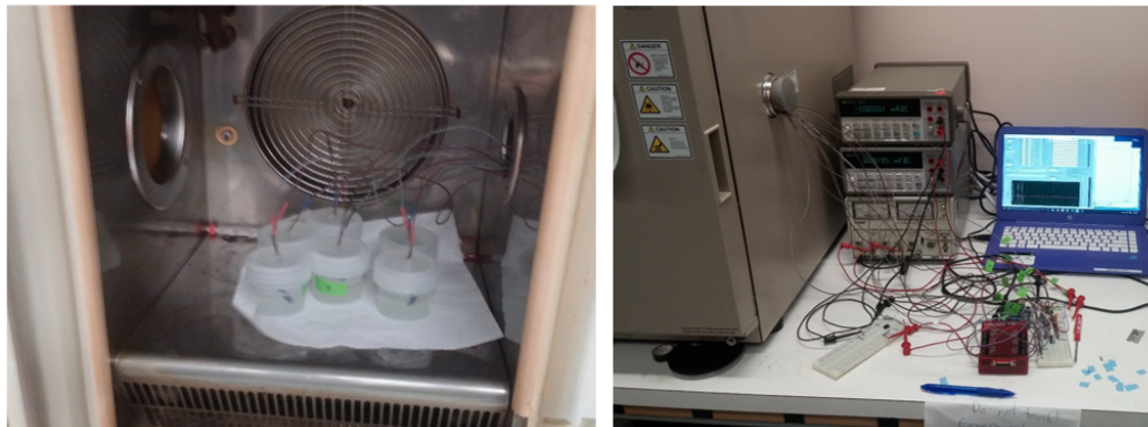
Figure A.8: Accelerated saline soak test setup, at 57 °C.
