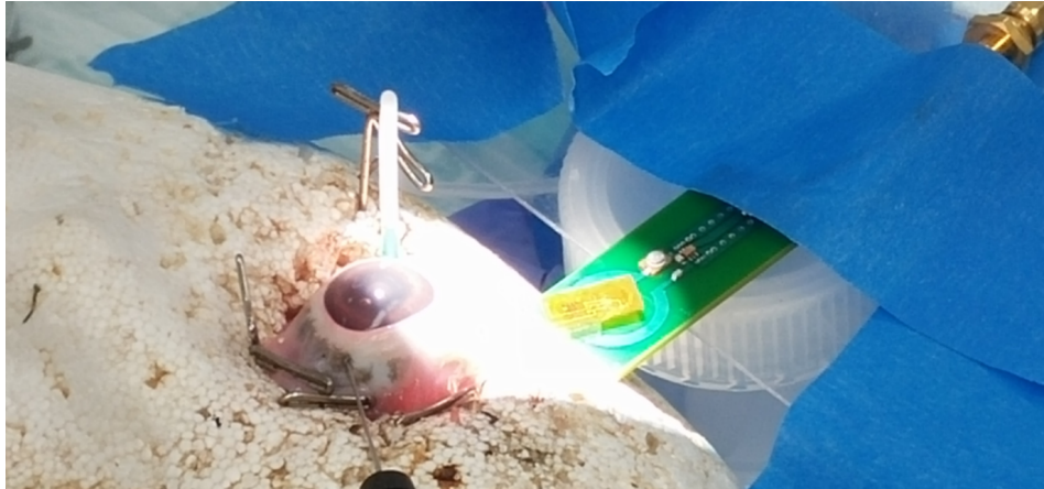
Figure 3.44: The implant is intended to be positioned on the eye as in Figure 3.43, but the readings were done with the implant body away from the eyeball laying flat on the reader coil. Earlier benchtop tests with the tube not inside the eyeball could get readings, but not in this particular experiment.
