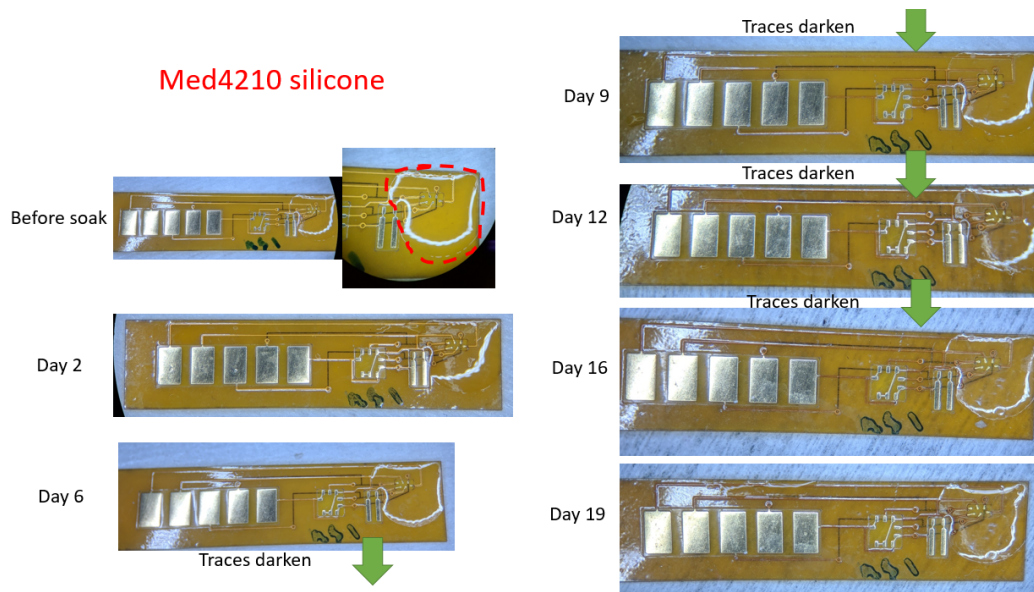
Figure 3.56: Med4210 as potting material (sample ns1, no wire bonds).
