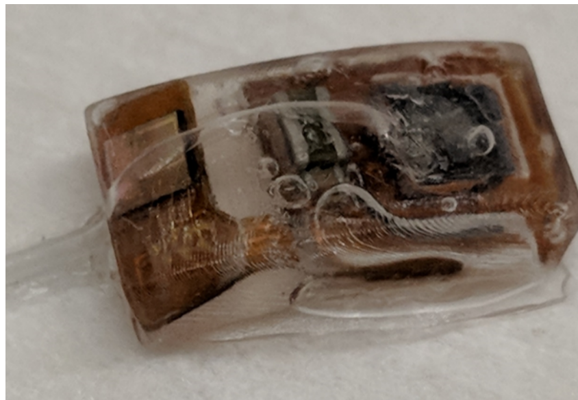
Figure 3.35: Cavity induced by excess IPA during removal of excess silicone.
