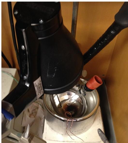
**Figure A.1:** Representative example of reaction setup using a 100-W Hg lamp. Ice is excluded for clarity.
