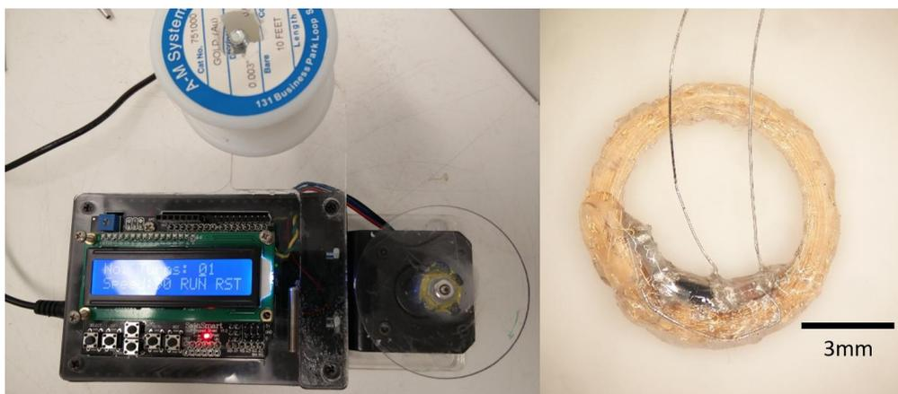
**Figure 5.16: Automatic coil winder.** (Left) Coil winder device. (Right) Active device electronics, V5. Coil surrounds the outside of the device. The coil is far more consistent in shape.
