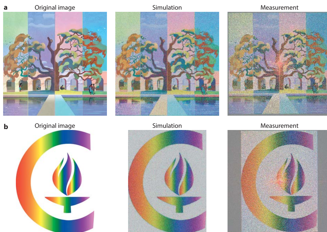
Figure 3.9: Simulation and measurement results a and b , The original target image along with simulated and measured polarization holograms converted to false-color images. Both holograms are about 30-degrees tall, corresponding to a diagonal NA of 0.36 for the holograms in panel a.
