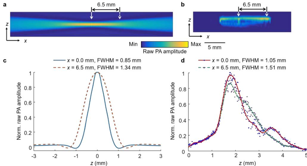
Figure 8. Quantification of elevational resolution of SIP-PACT. (a) Simulated acoustic focus field in the  $x$ - $z$  plane. (b) The PA image of a tungsten wire with a nominal diameter of  $50\ \mu\text{m}$ , projected on the  $x$ - $z$  plane. (c) The simulated line profiles of (a) at the center of
