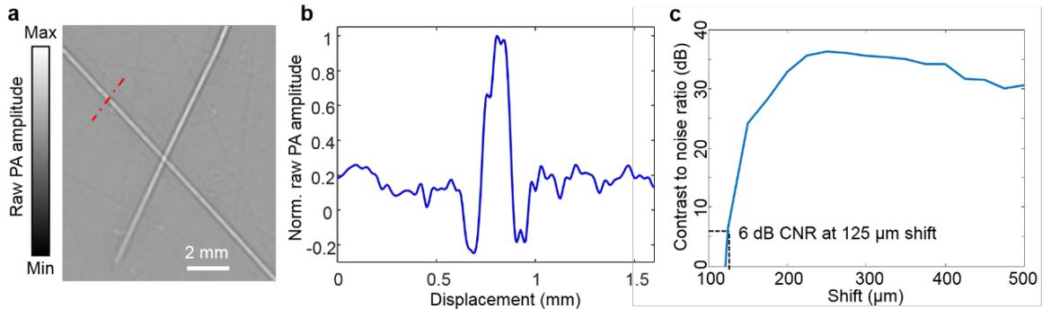
Figure 7. Quantification of the in-plane resolution of the SIP-PACT. (a) An image of two crossed tungsten wires, each with a nominal diameter of  $50\ \mu\text{m}$ . (b) The PA amplitude distribution along the red dash-dot line in (a). (c) The contrast-to-noise ratio (CNR) versus the shift in the sum of the original line profile shown in (b) and the shifted one. The in-plane resolution, defined as the shift corresponding to 6-dB CNR, is  $125\ \mu\text{m}$ .
