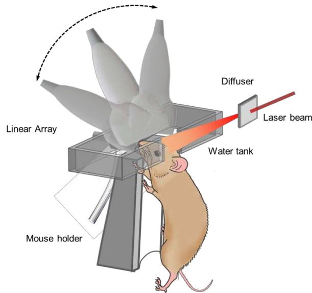
Figure 13 Schematic setup of linear-array based full-view PACT for mouse brain imaging.
