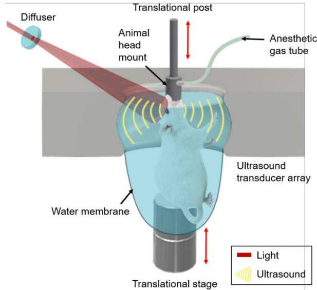
Figure 11. Setup for rat brain imaging. The rat head was mounted vertically during imaging and the light was obliquely delivered to the rat cortex.
