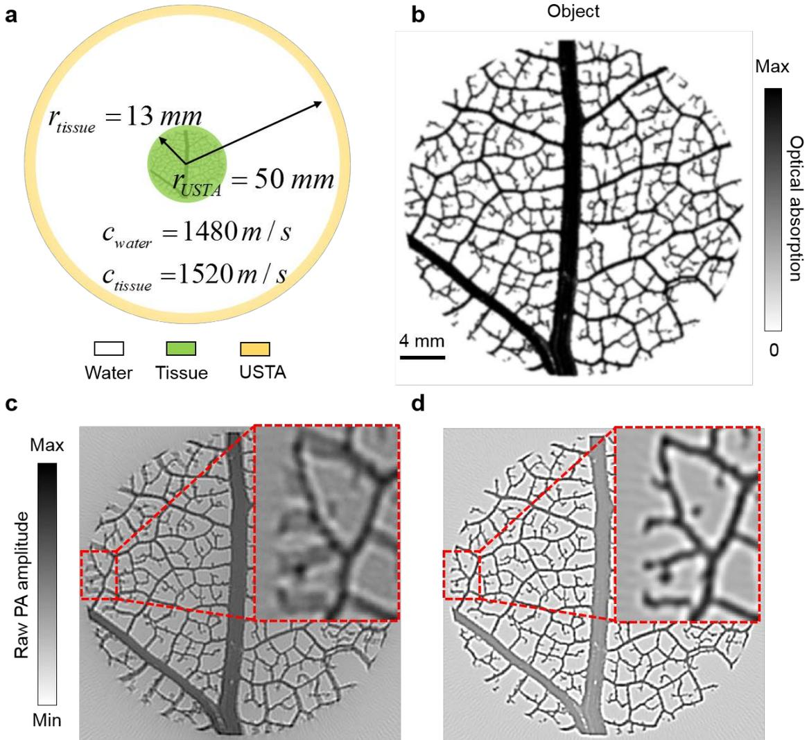
Figure 4. Numerical simulation results of dual-SOS reconstruction, forward data is generated by the k-Wave toolbox (<http://www.k-wave.org/>). (a) Schematic of the simulation. (b) The optical absorption distribution of the numerical phantom. Reconstructed images using universal back projection based on (c) single speed with  $v = 1489.8 \text{ m s}^{-1}$  and (d) dual speed with  $v_1 = 1480 \text{ m s}^{-1}$  (in water) and  $v_2 = 1520 \text{ m s}^{-1}$  (in
