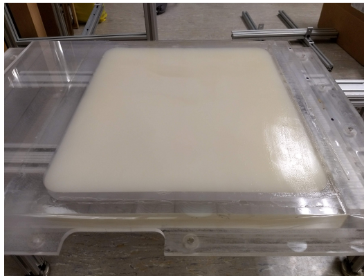
Figure 2.10: A finished gelatin sample. Note the sample pictured was dyed white for a DIC test. The gelatin used in the experiments was translucent.
