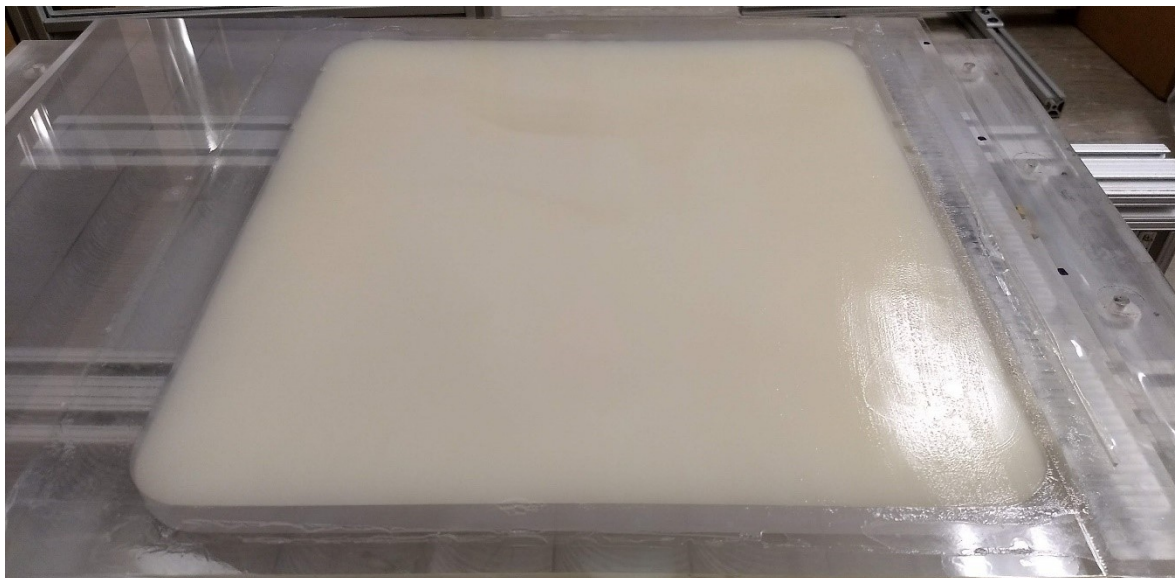
Figure A.4: Successfully fabricated gelatin sample, dyed white for a DIC test.
