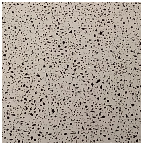
Figure 2.19: Photo of the speckle pattern generated with a fine mist water bottle and black India ink. The photo dimensions are 40 \times 40 \text{ mm}^2 .
