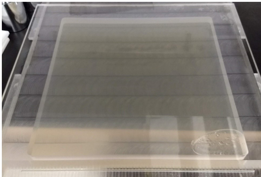
Figure A.2: Gelatin sample with non-Teflon cover on, bubble formed in corner due to curvature of cover plate.
