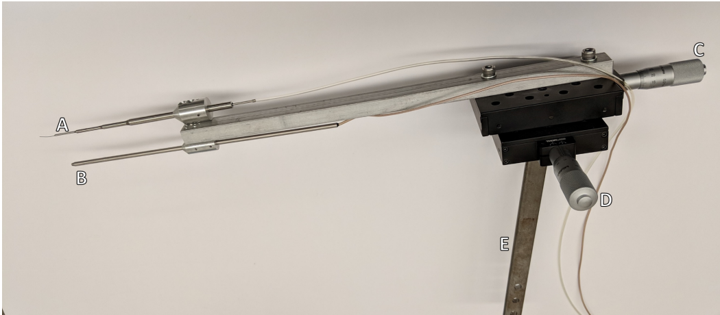
Figure 2.4: R1M traverse hot-wire probe setup. The pressure probe “A” is used for hot-wire calibration in the freestream. The hot-wire probe holder “B” holds a hot-wire probe (not shown). Linear stages “C” and “D” allow for streamwise and spanwise adjustment of the hot-wire probe. The post “E” extends below the roughness surface and is mounted to a powered traverse that allows wall-normal adjustment during the experiment.
