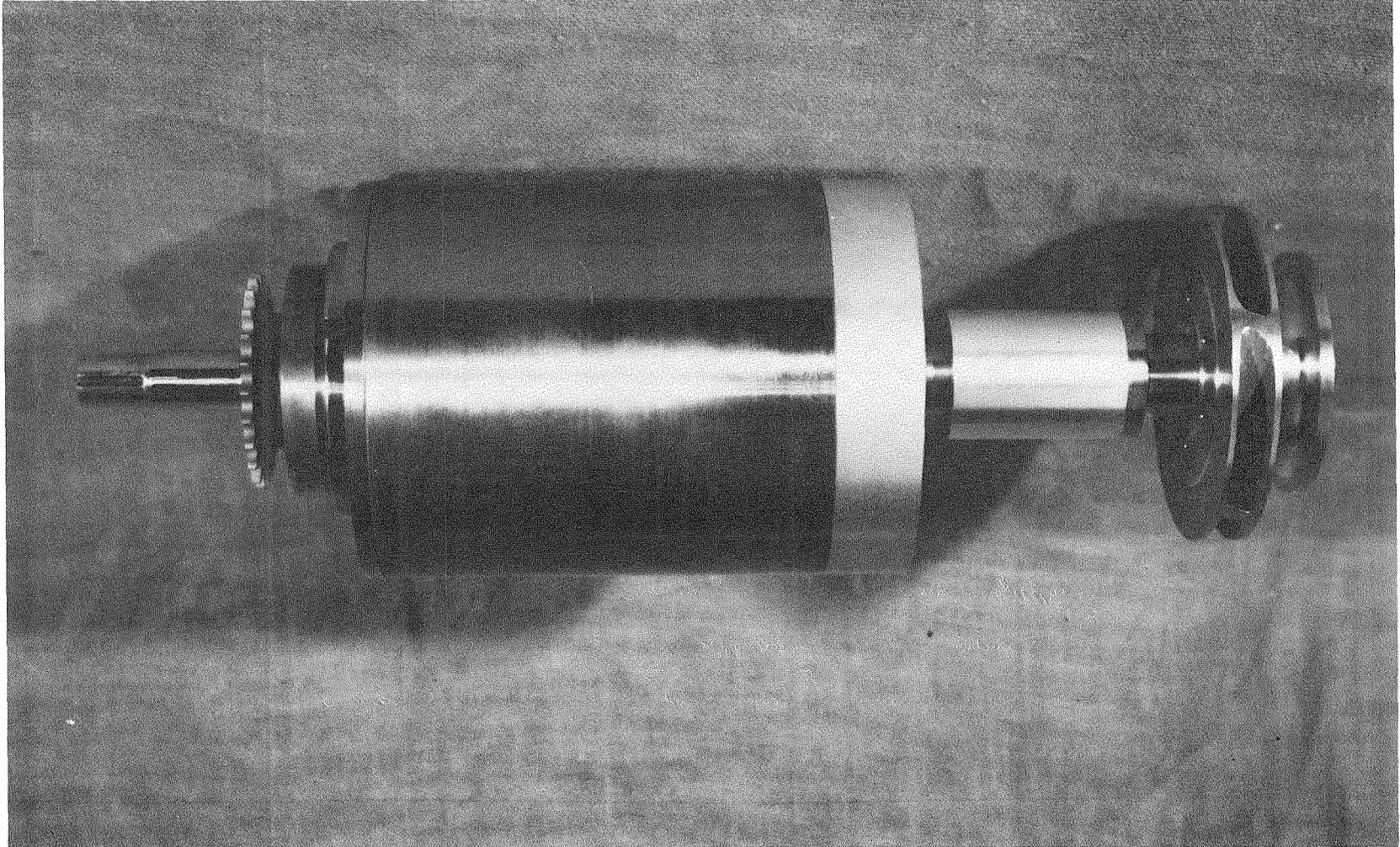
Fig. 3.5 Photograph of the eccentric drive disassembled from the Rotor Force Test Facility. Visible are (from left to right) the sprocket wheel, the main double bearing housing, a dummy replacing the actual dynamometer, and Impeller X mounted at the end of the drive shaft.
