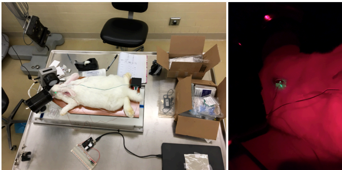
Figure 5.4: Experimental setup with rabbit, ERG, and LED contact lens used to determine the relationship between retinal illumination and rod dark current suppression.
