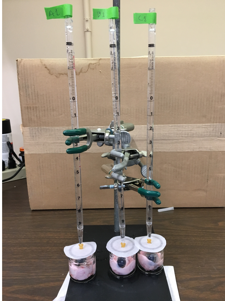
Figure 3.11: Experimental setup for permeation testing of enucleated porcine eyes with and without implants. Water columns of up to 28 cmH 2 O were inserted via syringe into the eyeballs and monitored over time to simultaneously record pressure and flow rate.
