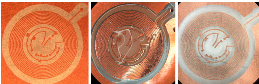
Figure 7.7: Copper on Parylene flexible circuit board fabrication. (Left) Photoresist patterned and developed on exposed copper, (Middle) midway through copper etching, (Right) Completed traces after stripping photoresist.
