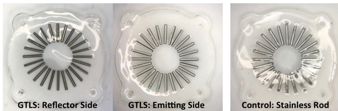
Figure 4.8: GTLS contact lens (left) and control lens (right) with suture holes to secure lens onto the rabbit eye for overnight studies.
