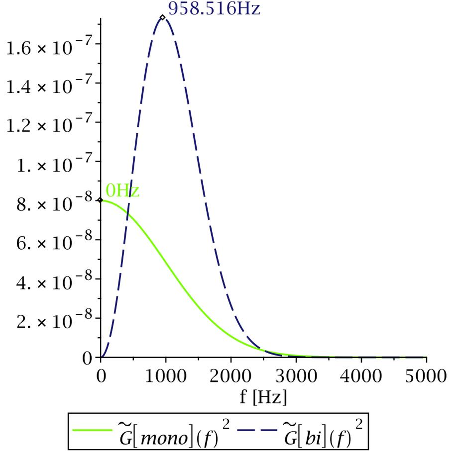
Figure 2.12: Plots of power spectral density for the monophasic Gaussian pulse  $\tilde{G}_{mono}(f, \varsigma_{mono})$  and the biphasic Gaussian pulse  $\tilde{G}_{bi}(f, \varsigma_{bi})$  used in this study
