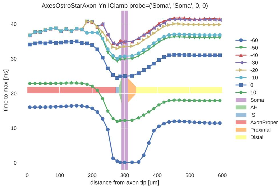
Figure 3.17: The time required for the soma to reach maximum membrane voltage (y-axis in  $\mu\text{s}$ ) when a 0.1 ms square current pulse is injected at that distance from the axon tip (x-axis) with the current necessary (see Fig. 3.16) to reach the specified membrane voltage (see legend).
