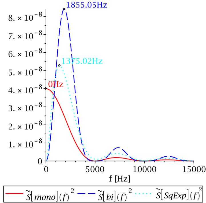
Figure 2.10: Plots of power spectral density for monophasic square pulse ( $\tilde{S}_{mono}^2(f, w = 200 \mu s)$ ), biphasic square pulse ( $\tilde{S}_{bi}^2(f, w = 200 \mu s)$ ), and biphasic square exponential ( $\tilde{S}_{SqExp}^2(f, w = 200 \mu s)$ ).
