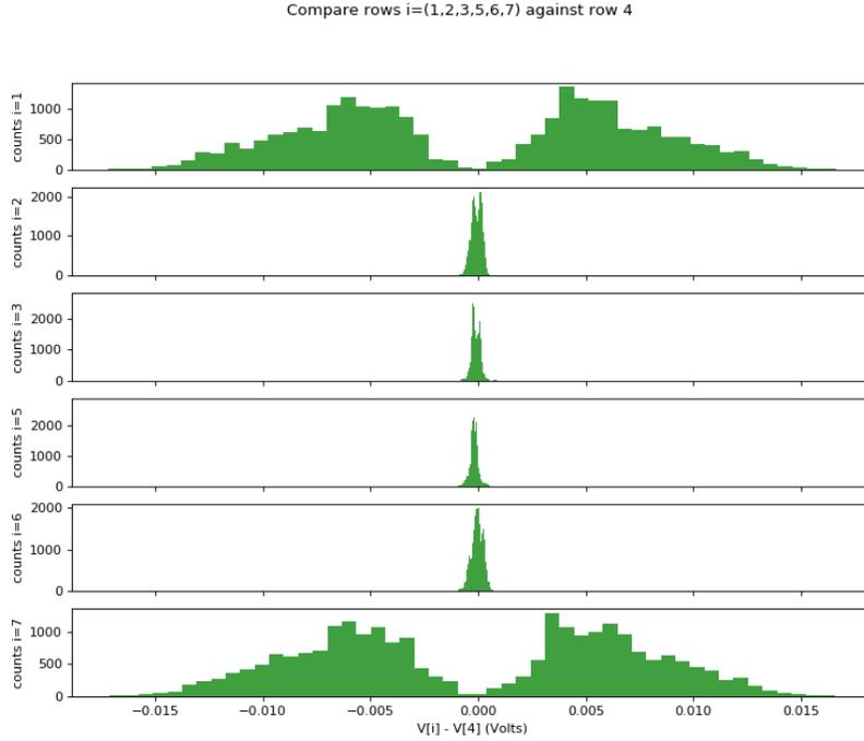
Figure 2.15: Comparison of combination translations along the  $\hat{z}$  axis. Note the edge effects in row 1 and 7. The histogram includes all three single row combinations (ANpBNn, ANpCNn, BNpCNn) (where  $N$  is the row number) and stationary simulations run at  $f_{\text{mono}}^{\text{max}} = 0$  Hz and  $f_{\text{bi}}^{\text{max}} \approx 958.5$  Hz.
