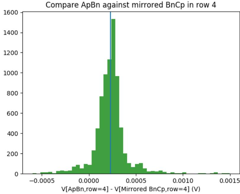
Figure 2.16: Comparison of combination ( $A4 = 1V, B4 = -1V$ ) with mirrored combination ( $C4 = 1V, B4 = -1V$ ). The mean difference is 0.229 mV (indicated by vertical line) and the maximum difference was 1.49 mV. The histogram includes stationary simulations run at  $f_{\text{mono}}^{\text{max}} = 0$  Hz and  $f_{\text{bi}}^{\text{max}} \approx 958.5$  Hz.
