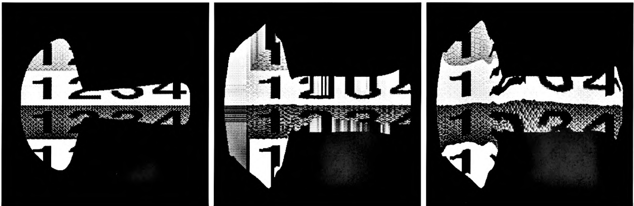
Figure 4.4: Left: Texture map if range data were noiseless, and the model matched it exactly. Middle: Nearest-Neighbor when model is translated and has noise added. Right: Texture map using fractional mappings. □
