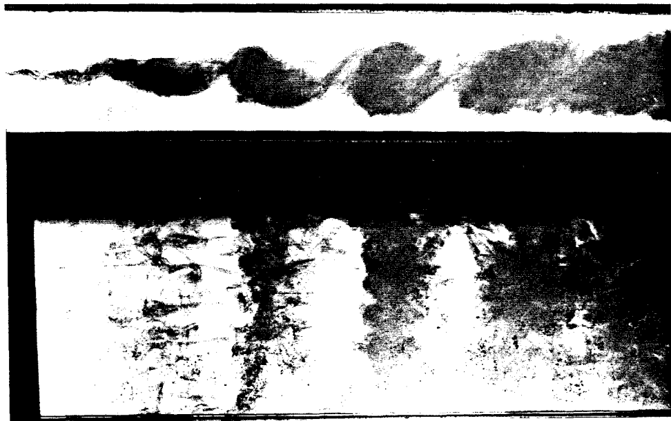
Figure 3.19 : Product Thickness and Growth Rate from Absorption Measurement -- Low Reynolds Number , F = 1.8 \text{ Hz}
