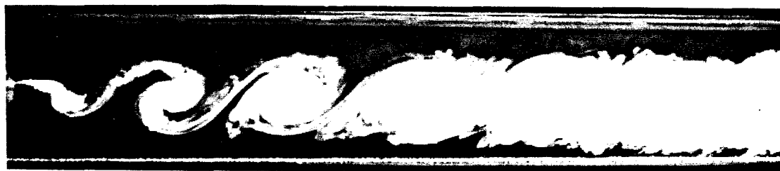
(c) F = 8 \text{ Hz} , F/F_0 = 0.13 , \lambda = 6 \text{ cm} \longleftrightarrow
