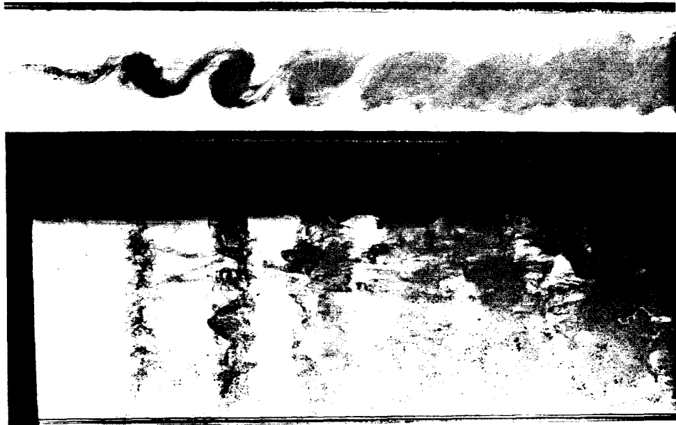
Figure 3.20 : Product Thickness and Growth Rate from Absorption Measurement -- Low Reynolds Number , F = 2.6 \text{ Hz}
