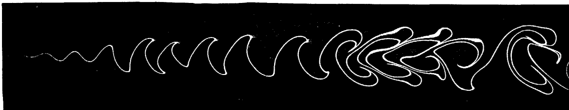
(b) Reacting L.I.F. Cross-section. Scale different than (a).
