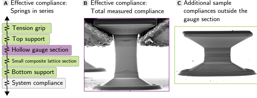
Figure 3.3: Displacement and strain for the hollow gauge section only can be obtained by subtracting the contribution of the additional compliance from the effective compliance recorded by the nanomechanical instrument.
