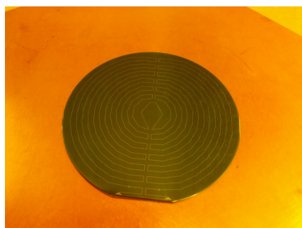
Figure 7.16: Left: an example of a 25-nm Nb feedline-only device. A number of these inspected very well, but upon testing 50% had very poor transmission. Right: a plot of the magnitude of the complex transmission of two devices that inspected identically well. Device 1 (blue) had very poor transmission and would be unusable in a device with MKIDs. Device 2 (Orange) does have a few residual RF resonances, but there is enough flat frequency domain that the majority of MKIDs on such a device could be found and fit.
