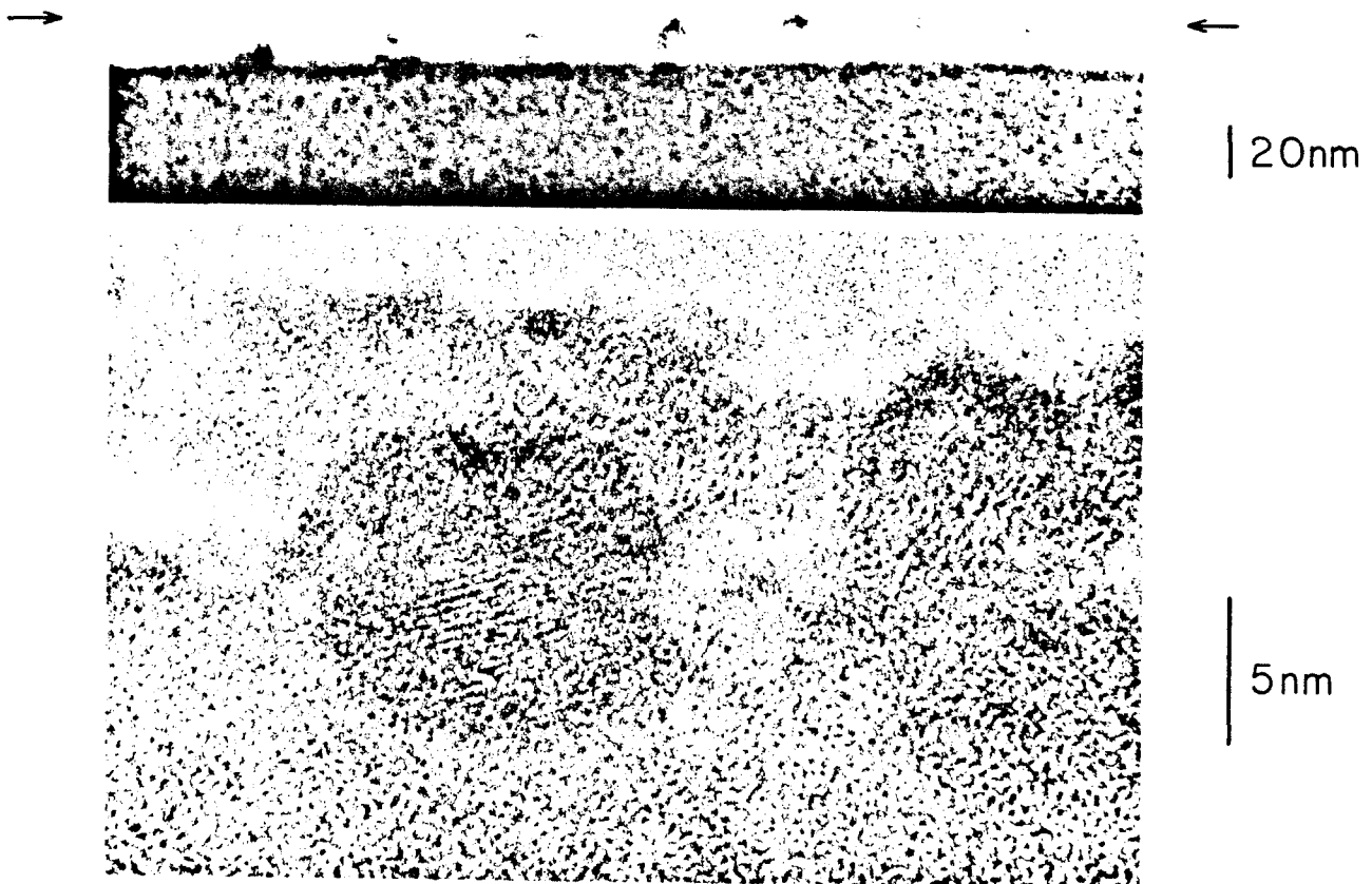
Figure 8b. (Top) TEM image for irradiated Ti/SiO 2 sample after etching. The arrows indicate the surface of the SiO 2 .
