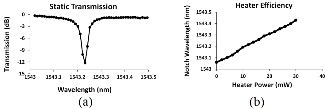
Figure 9.21: (a) Measured steady-state transmission of the ring near a notch (b) tunability of the ring
