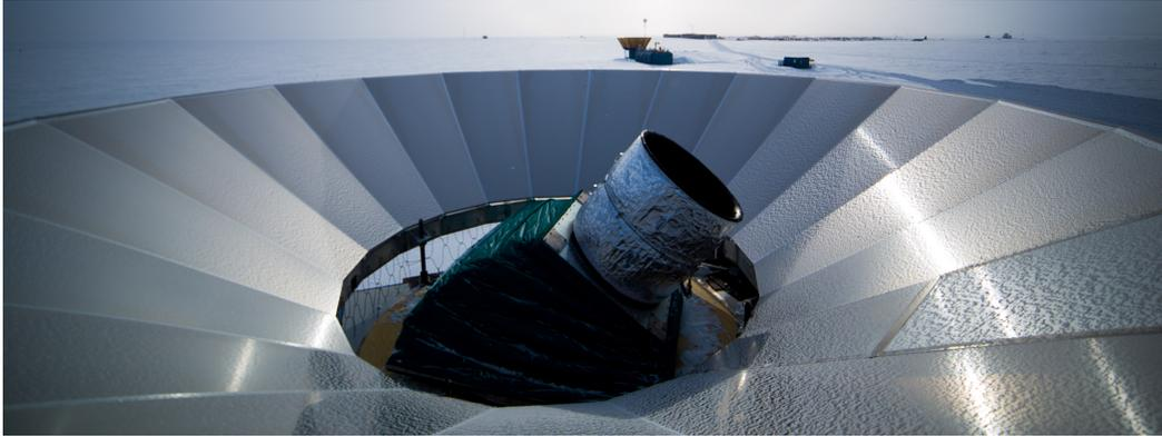
Figure 3.2: View of BICEP3 from the roof of DSL, showing the green insulating boot, comoving forebaffle, and reflective ground shield. The forebaffle intercepts radiation  $> 14^\circ$  from the telescope boresight. The larger *Keck Array* ground shield is visible in the background and the main Amundsen-Scott station extends along the horizon.
