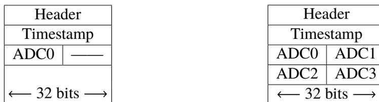
Figure 5.4: The anatomy of a single hit, as prepared by the FPGA on the FEB for single(multi)point timing on the left(right). Due to the overhead of the header and timestamp to specify the channel and time of the hit, including the three additional ADC values for offline fitting only increases the size of the hit by a third.
