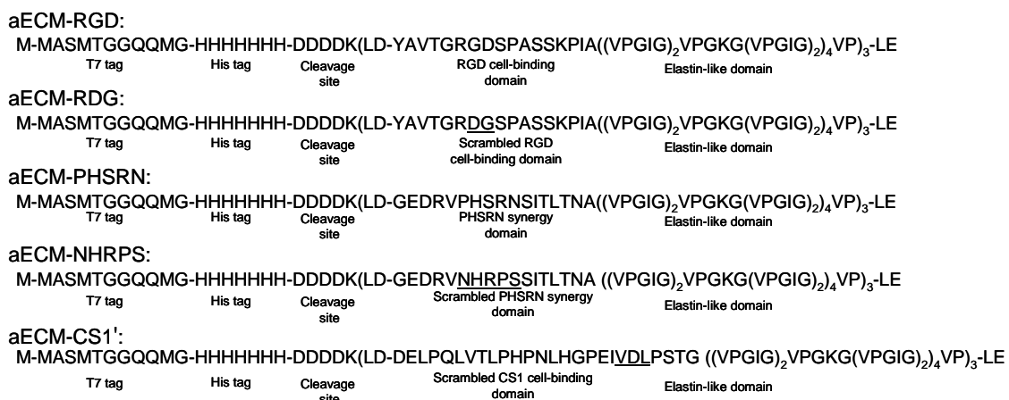
Figure 2.1 Artificial extracellular matrix protein sequences. The bioactive domains include an RGD cell-binding domain, a scrambled RDG sequence, a PHSRN synergy site, a scrambled NHRPS sequence, and a scrambled CS1' sequence. The proteins also include a T7 tag, heptahistidine tag, enterokinase cleavage site, and elastin-like repeats containing lysine residues that serve as crosslinking sites.
