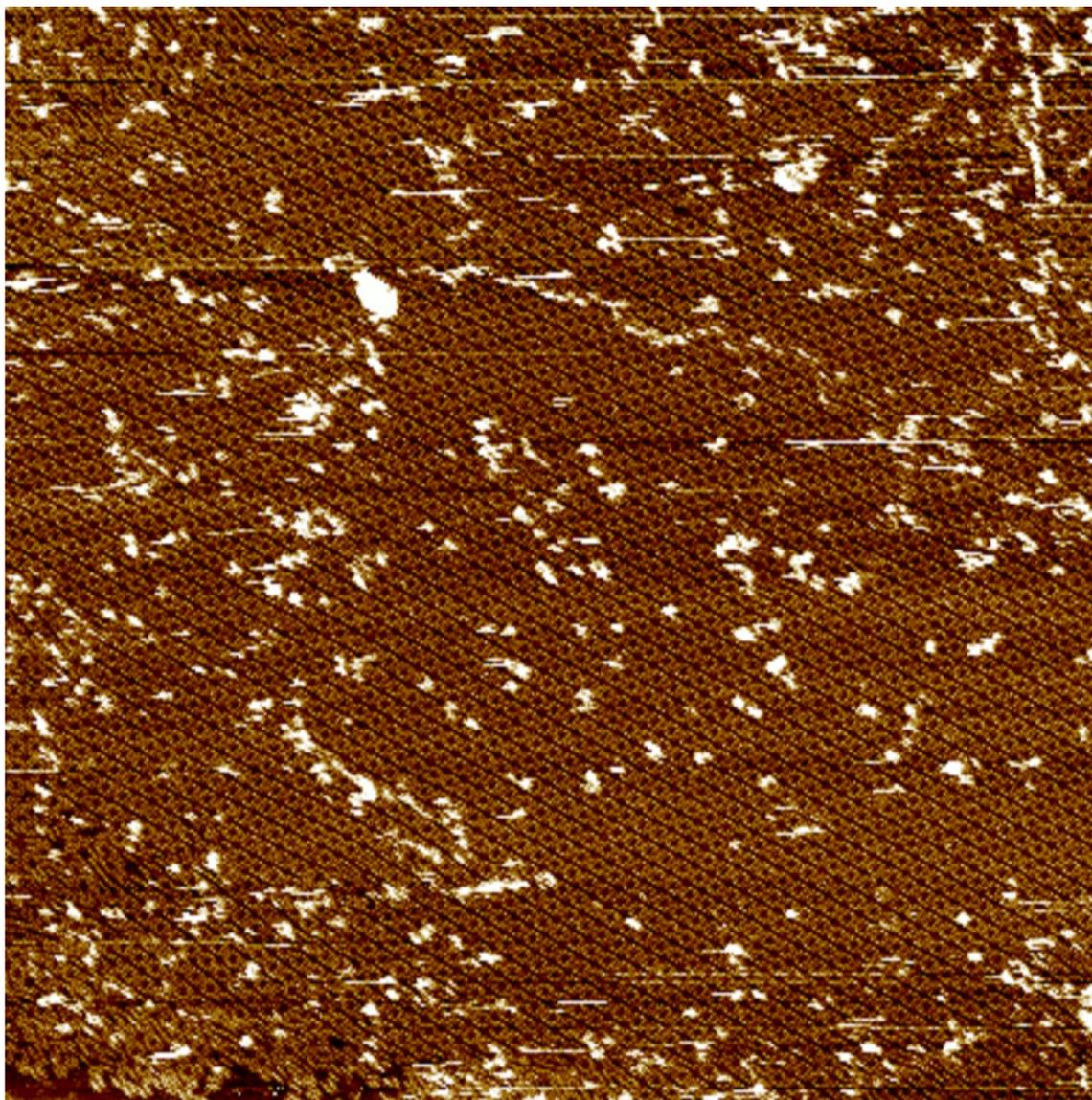
Figure 3.6a. 7 by 7 um AFM image showing part of a crystalline domain of unbounded tiles with double-stranded surface modifications forming circle patterns.
