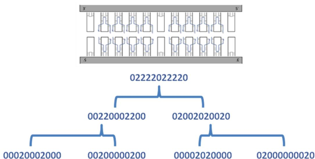
Figure 4.5. **Edge rule.** The edge rule for splitting staples in each stage. 0s represent the absence of a staple (open M13). 2s represent staple that is either truncated or extended by two nucleotides. Edges are split evenly in each stage and are palindromic. Each 2 in the second to fifth digits in each code corresponds to an indentation or bump on a tile edge shown in 4.2(c).
