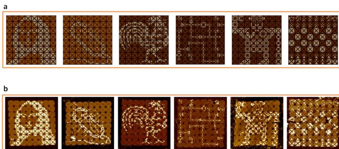
Figure 4.20: **Software aided automatically mixed experiments.** **a**, Design diagrams displayed in mock AFM colors predictive of the design's appearance on AFM. **b**, The actual AFM images: a Mona Lisa, a bacteria scale bacteria, a rooster, a photoreceptor circuit [19], a DNA robot (drawing), and a chess game.
