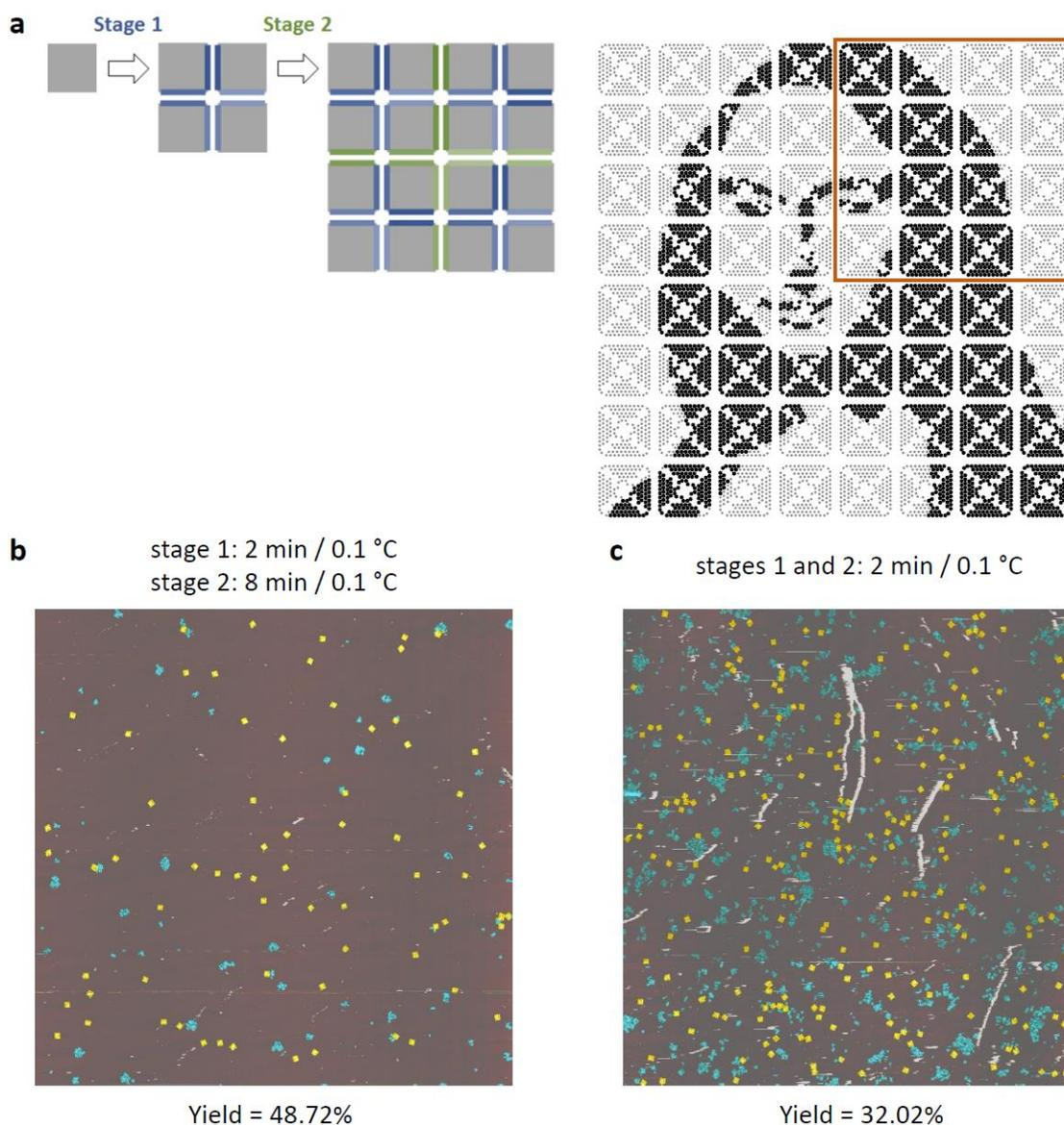
Figure 4.12. **Annealing time per stage.** **a**, Design diagram of a 4 by 4 quadrant of an 8 by 8 array with a Mona Lisa pattern. **b**, AFM image of the quadrant annealed for 2 minutes per 0.1 °C in stage 1 and 8 minutes per 0.1 °C in the stage 2. **c**, both stages were annealed 2 minutes per 0.1 °C
