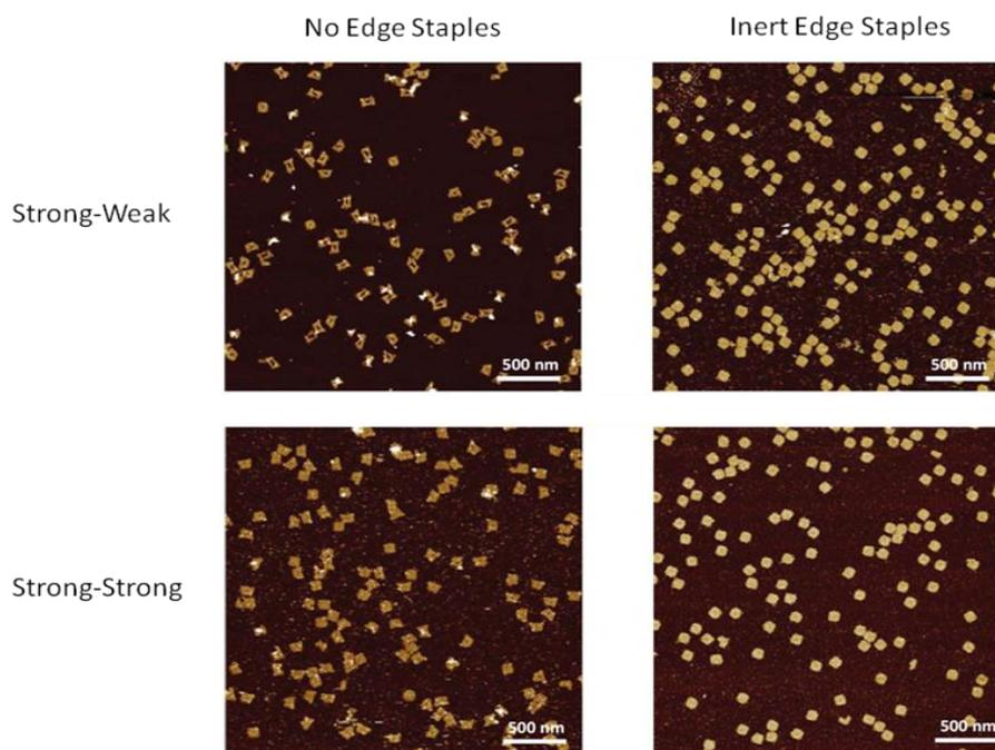
Figure 2.5: **AFM images of strong-weak and strong-strong bridges without edge staples or with a full set of inert edge staples.** Without edge staples, the weaker bridges allowed the tiles to rip apart at the seams. The strong-strong tiles were better able to hold the seams closed on imaging. With inert edges, the tiles were fairly intact in both designs.
