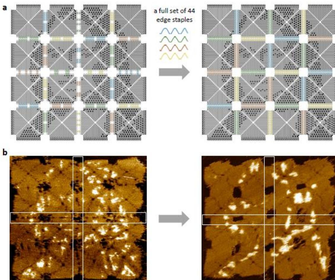
Figure 4.18. **Strengthening origami arrays after fractal assembly a**, design diagram. **b**, AFM of 4 by 4 array before and then after strengthening. The white box highlights the most obvious changes on the edges (4 staples per edge on the left to 11 staples per edge on the right).
