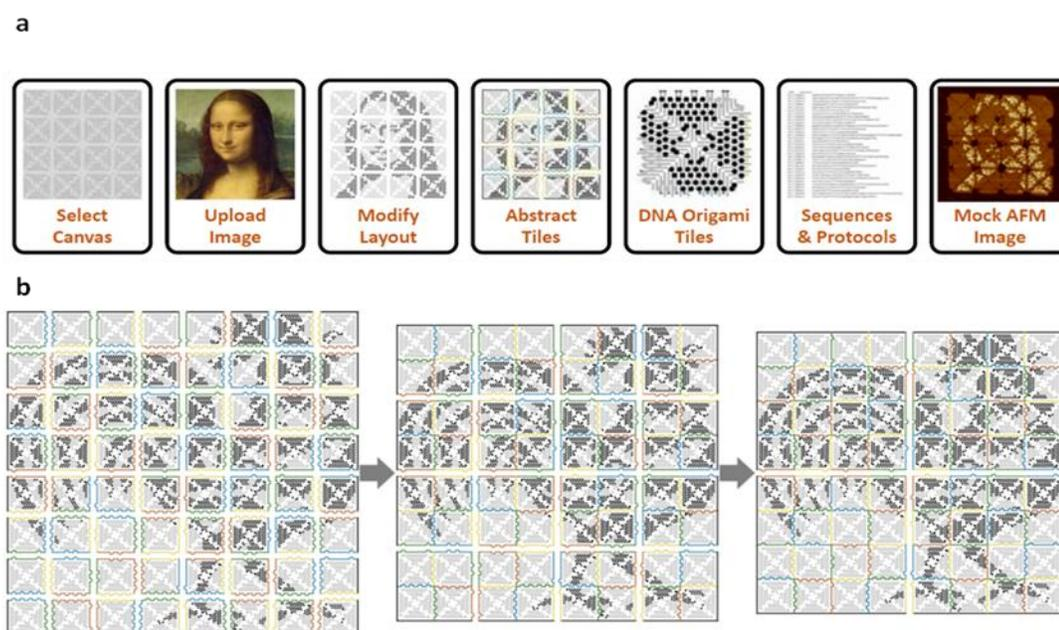
Figure 4.19. **Drawing and display options of the FracTile Compiler.** **a**, main options available with the software [18]. From left to right: canvas size selection, image uploading, image modification options, display abstract tiles showing the Fractal Assembly process, display detailed DNA origami tiles showing edge configurations, display mixing protocols, show image with mock AFM colors. **b**, Abstract Tile diagram display for a rooster image.
