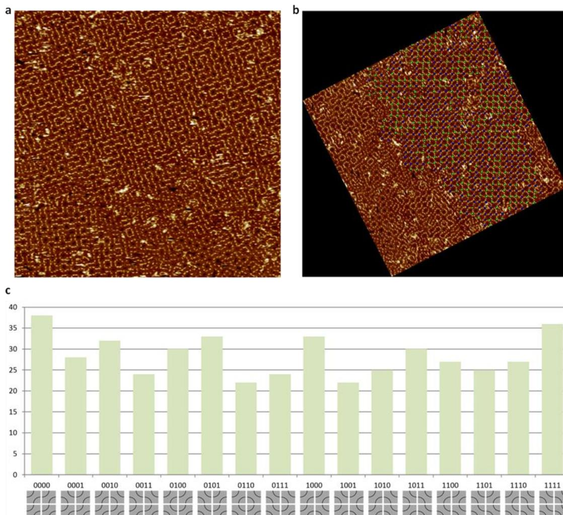
Figure 3.8. **Analysis of tile orientations of arc tiles forming a loop maze pattern on an array.** **a**, Representative AFM image showing arc tiles in two orientation resulting in a loop pattern. **b**, rotated image with the tile orientation marked with blue or green dots. **c**, Counts of all 16 possible two by two local neighborhoods.  $n=456$  neighborhoods. Each pattern appears  $28.5 \pm 4.9$  times ( $6.25\% \pm 1.07\%$ ).
