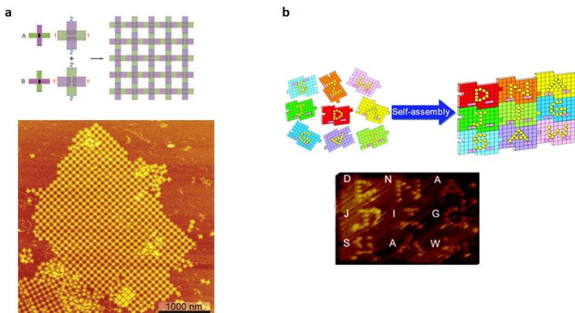
Figure 1.4. **Scaling up DNA origami.** **a**, periodic array of DNA origami tiles. **b**, three by three array of DNA origami tiles.
