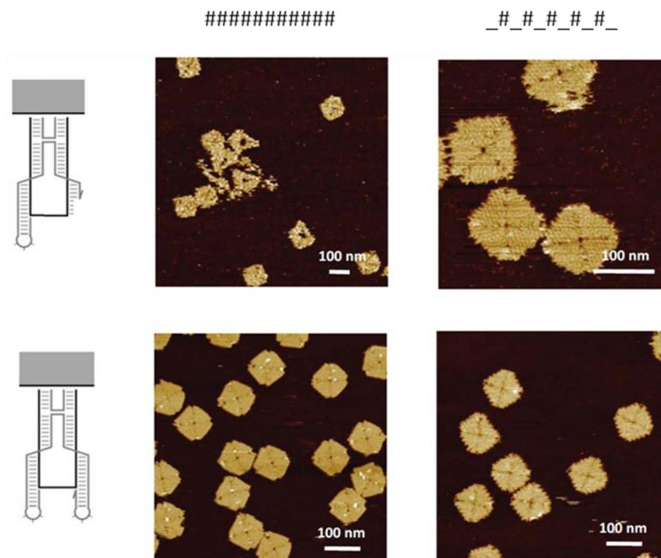
Figure 2.7: **Hairpin capped edge staples.** '#' represents the presence of a hairpin edge staple whereas '\_' is the absence of any edge staple at that location. Four designs: 5' hairpin and 3' truncation for each edge staple in either a full edge set (top-left) or spaced layout (top-right), a hairpin on both the 5' and 3' end of edge staples in either a full edge set (bottom-left) or spaced layout (bottom-right).
