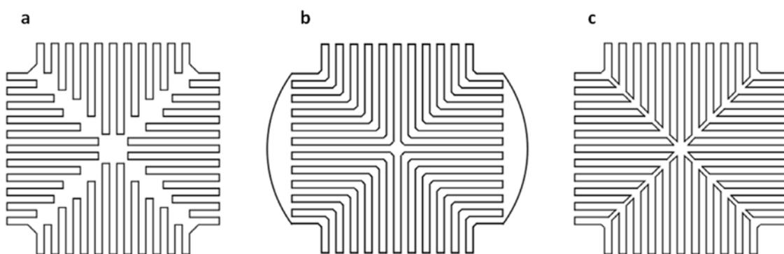
Figure 2.2: **Scaffold paths for a square DNA origami tile.** **a**, scaffold path fills each of the four triangles within the tile with internal crossovers at the end of each helix row. **b**, scaffold path fills each square corner quadrants within the tile. **c**, scaffold path fills each of the four triangles within the tile with scaffold loops connecting helices within the interior of the tile.
