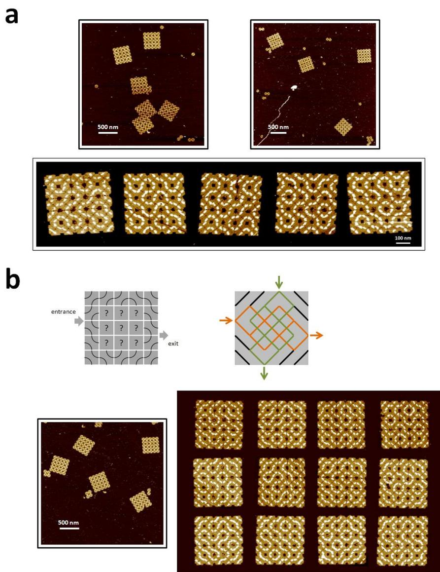
Figure 3.20. **Random loops and mazes on the entire or part of a 5 by 5 finite array.** **a**, Random loops and mazes on entire 5 by 5 arrays. The bottom image is composed from 5 separate zoomed in AFM images. **b**, Designed mazes with fixed orientation of exterior tiles and random orientation of interior tiles. The right image is composed of 12 separate zoomed in AFM images.
