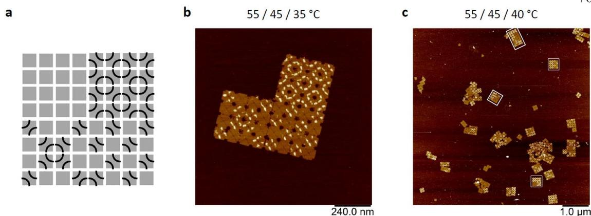
Figure 4.7. **Annealing temperature.** **a**, Design diagram of an 8 by 8 fractal array. Each quadrant has a unique pattern. **b**, AFM image of an incomplete 8 by 8 array, but with correctly formed quadrants. The annealing schedule was 55, 45, and 35 °C to 20 °C for each stage respectively. **c**, AFM image of scrambled and incomplete arrays. The last stage anneal was raised to 40 to 20 °C. A few scrambled structures are outlined.
