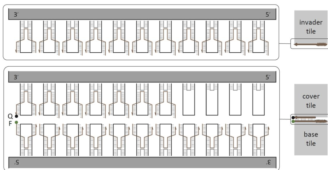
Figure 5.4. **Edge design of tiles.** All domains are formed from staples interacting through sticky ends and stacking bonds. Open toeholds are formed by removing staples in the opposite staple locations within the dimer complex.
