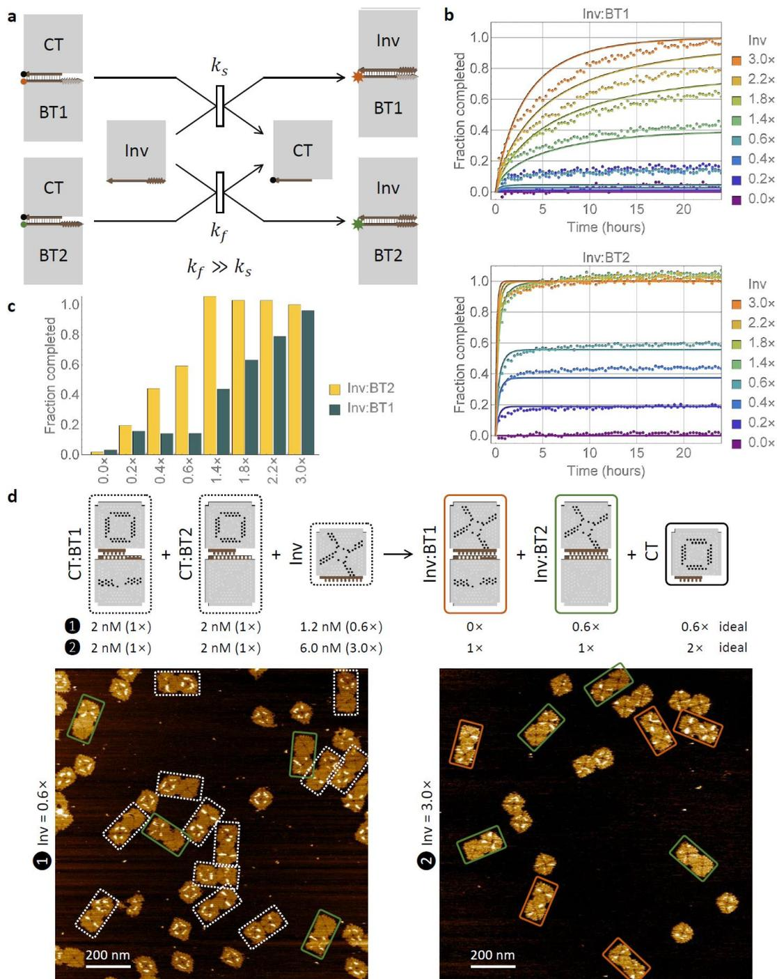
Figure 5.7. **Competitive reconfiguration.** **a**, tile abstract diagram. Invader tile can react with either dimer CT:BT1 or dimer CT:BT2 with different kinetics. **b**, fluorescence kinetics data for the two dimers at 2nM with variable amounts of invader tile added. **c**, Completion levels **d**, Origami diagrams and AFM images of two invader concentrations. Left: 1.2nM, right: 6nM. Dotted outlines are incomplete structures. Solid colored outlines are complete reactions.
