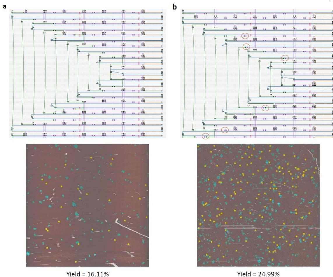
Figure 4.10. **Bridge and interior staple redesign for increased continuous addressable surface area.** **a**, Original Cadnano [10] diagram with 112 pixels and a formed 4 by 4 array (same design as in 4.9 (c and d)). **b**, New Cadnano design with 136 pixels. Correct structures are colored yellow, with the rest colored blue.
