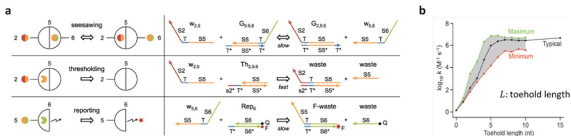
Figure 5.5. **DNA circuits and rate tuning.** **a**, Simple DNA building blocks using strand displacement and its rates, capable of scaling to large digital logic circuits [15]. **b**, Variable rate of strand displacement over several orders of magnitude.
