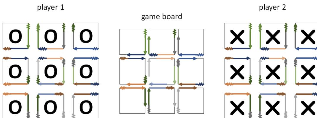
Figure 5.10. **Design of Tic-Tac-Toe game board on a three by three array.** Toeholds are marked with jagged colored lines. Branch migration domain are solid colored lines. See Appendix A for detailed design diagram.
