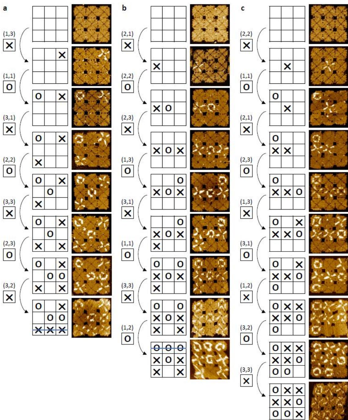
Figure 5.12. Full games of Tic-Tac-Toe based on tile displacement to reconfigure the game board. For each game played, the abstract diagram is shown on the left and an AFM image of that move on the right.
