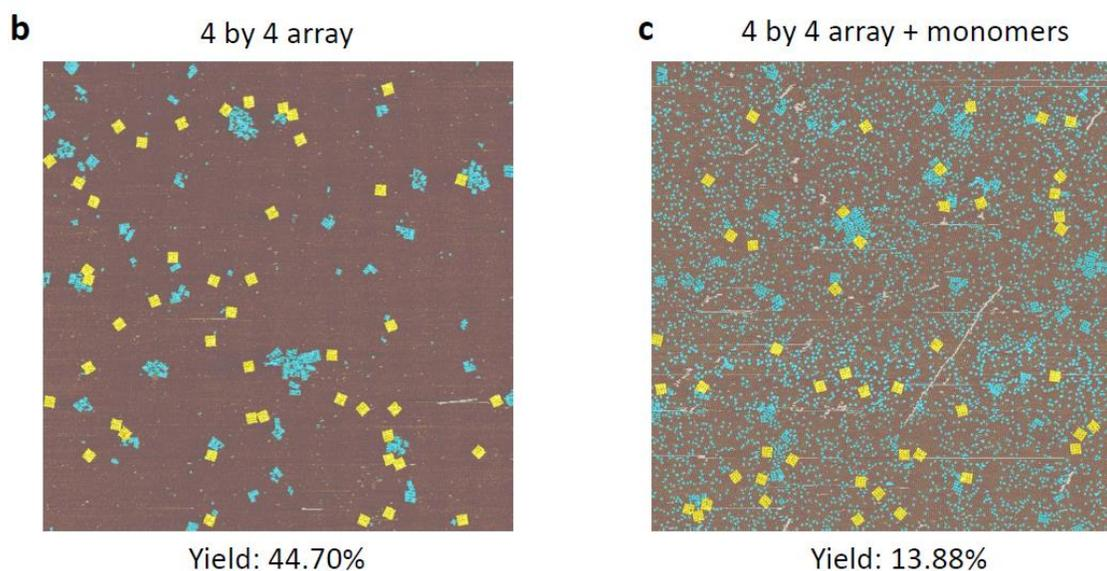
Figure 4.14. **Assessing accuracy of AFM-based yield estimation.** **a**, Three case scenarios for yield estimation. **b**, Yield of plain 4 by 4 arrays. **c**, Yield of the same plain 4 by 4 arrays mixed with monomers. The yield is less than half.
