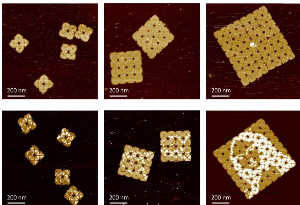
Figure 4.13. **Experimental demonstration of fractal assembly.** AFM images of 2 by 2, 4 by 4, and 8 by 8 arrays with either no surface modifications (top row) or a Mona Lisa pattern (bottom row)
