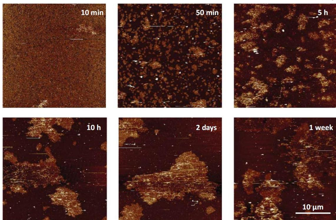
Figure 3.5. Representative AFM images of unbounded arrays with increasing anneal time.
