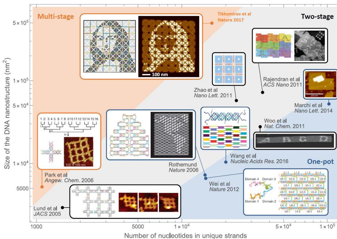
Figure 4.0: **The development of arbitrarily patternable two-dimensional DNA structures.** Log-log plot comparing the size of a DNA structure against the required number of nucleotides in unique strands in that structure.
