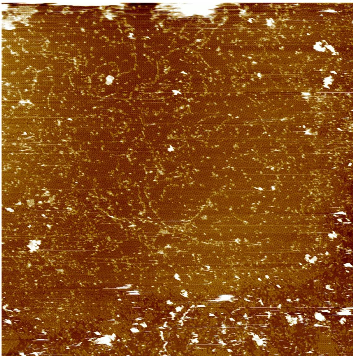
Figure 3.6b: A 16.2 by 16.2  $\mu\text{m}$  AFM image showing part of a crystalline domain of unbounded tiles with double-stranded surface modifications forming circle patterns. There exists some defects at this scale. Zoom in to see the circle patterns showing the domains.
