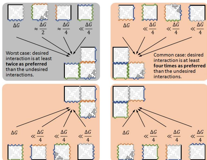
Figure 4.8: **Desired and undesired interaction preference.** The worst case maintains a desired reaction at least twice as preferred as undesired. Normally, the desired is at least four times more preferred. In subsequent stages, this gap between desire and undesired generally increases due to geometric spacing.
