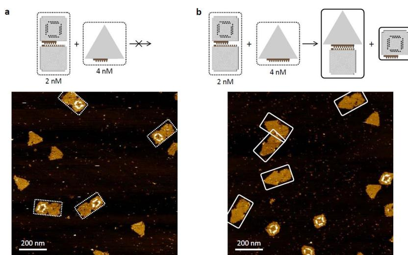
Figure 5.3. Triangle shaped invader tile reconfigures a square-square dimer complex into a triangle-square dimer complex. **a**, Triangle without a proper toehold does not react. **b**, Triangle with a toehold reacts.
