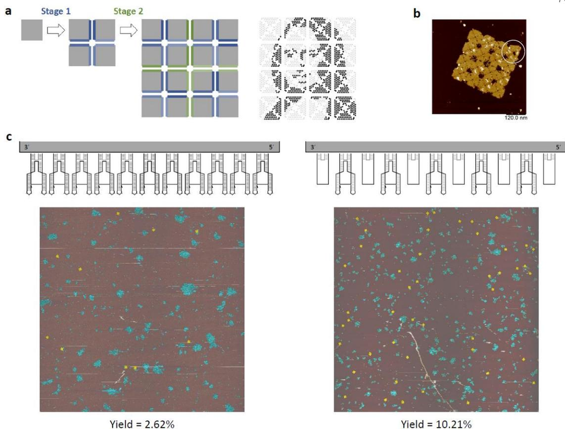
Figure 4.9. **Inert edges.** **a**, Design diagram for (c). **b**, four by four array from a low yield quadrant showing a deformation. **c**, Edge diagram and AFM images for eleven and five double-hairpin edge staples per edge at the exterior of the array. Correct structures are colored yellow, with the rest colored blue.
