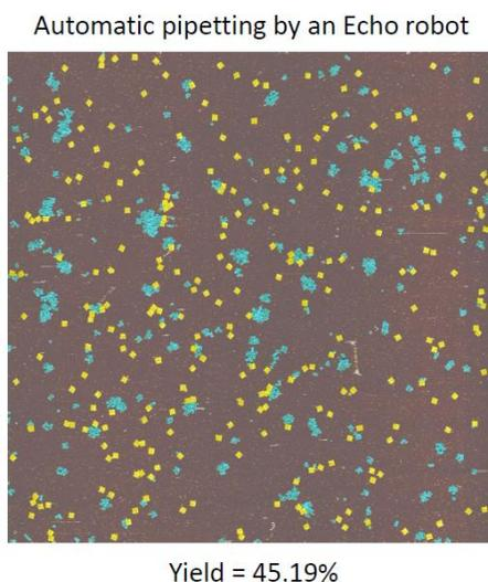
Figure 4.11. **Automatic liquid handler.** Same 4 by 4 design as in 4.10(b). Automatically mixed by an Echo 525 liquid handler. Correct structures are colored yellow, with the rest colored blue.
