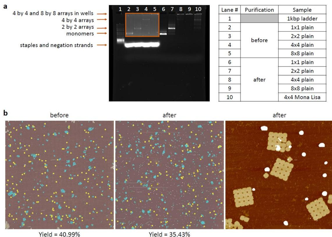
Figure 4.17. **Spin-filter purification.** **a**, 1 by 1 (monomer) to 8 by 8 arrays before and after purification. 0.5% agarose gel, ran at 80 mV for 2 hours. The contrast was increase in the orange box to show bands at low concentrations. **b**, AFM images of 4 by 4 arrays pre and post purification.
