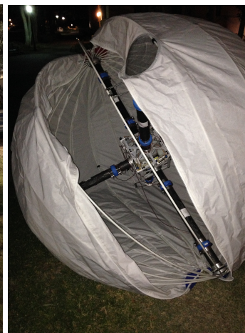
(c) Moball with open shell, displaying internal hardware.
