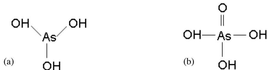
Figure 2.1. Structures of (a) arsenous acid, or arsenite; pK_{a1} = 9.23 , pK_{a2} = 12.13 , pK_{a3} = 13.4 ; and (b) arsenic acid, or arsenate; pK_{a1} = 2.22 , pK_{a2} = 6.98 , pK_{a3} = 11.53 .
